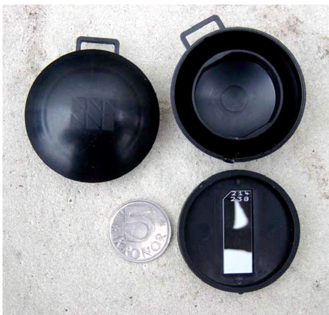
Figure 4. The alpha-track film detector used in the Estonian National Radon Survey. The detector holder on the right is open to show the plastic film used. The detector holder is closed during the measurement. Radon gas seeps into the detector through a thin slot between the lid and the bottom of the detector holder.
