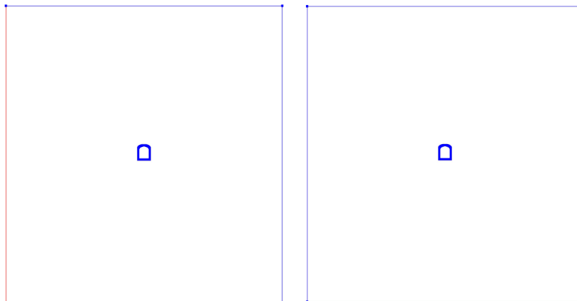
Figure 61. Left and bottom boundaries are selected as roller boundaries.
