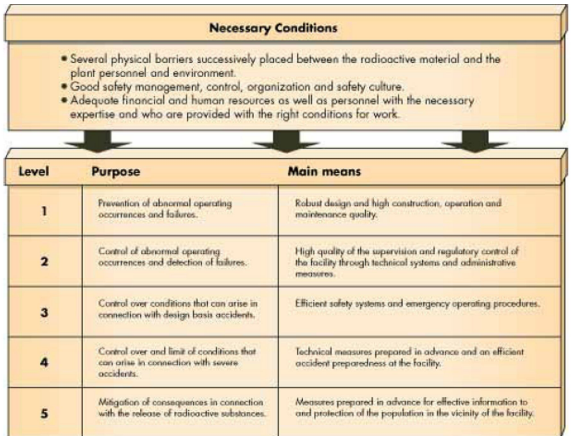
Figure 1. The necessary conditions for a defence in depth system and the different levels of the system
