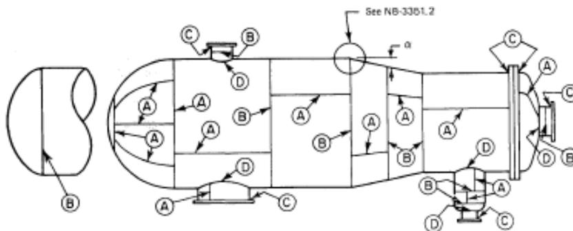
**Figure 6:** Figure NB-3351-1: Welded Joint Locations Typical of Categories A, B, C and D
