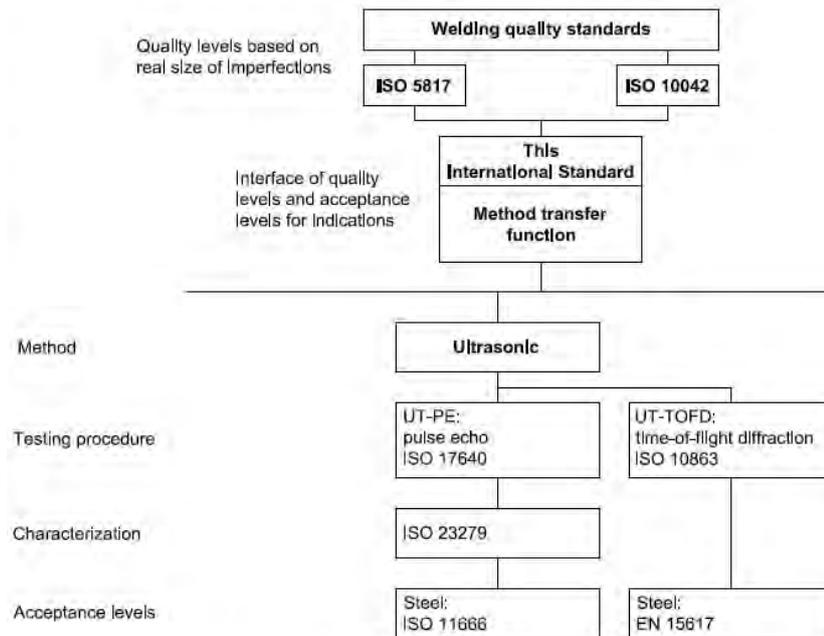
**Figure 3:** Graph of standard context for ultrasonic methods
