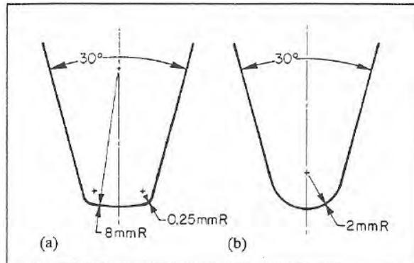
**Figure 4:** Schematic drawing of the (a) ASTM (8 mm radius) and (b) ISO (2 mm radius) striker
