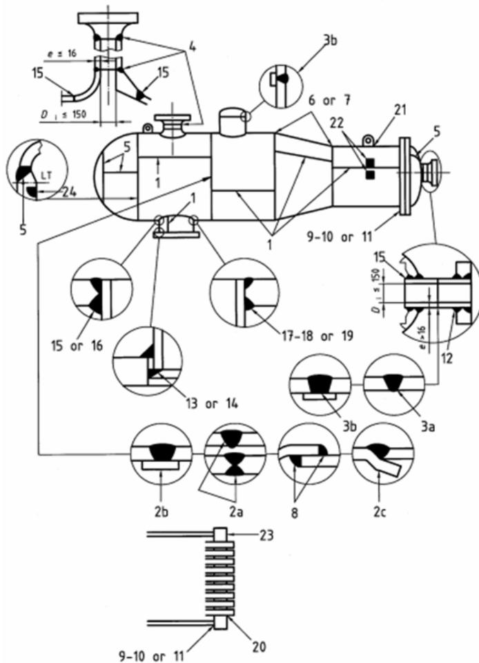
**Figure 7:** Figure 6.6.2-3 – Type of welds
