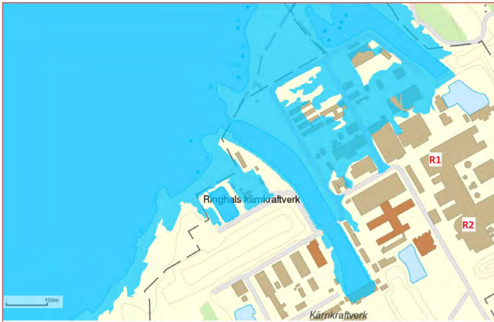
Figure 1-10. Flooding at a postulated sea level rise of 300 cm (RH 2000). The picture is a slightly edited version of the original in [6] as the R1 and R2 reactor buildings have been marked for reference.
