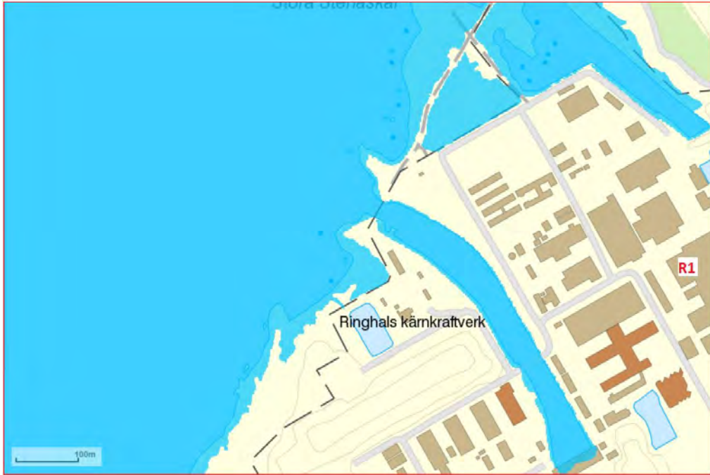
Figure 1-9. Flooding at a postulated sea level rise of 200 cm (RH 2000). The picture is a slightly edited version of the original in [6] as the R1 reactor building has been marked for reference.
