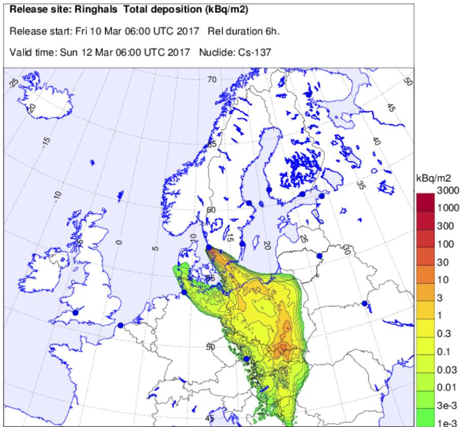
**Figure 1.** Example of outcome from an atmospheric dispersion calculation. The illustration is based on a fictitious release of Cs-137 from the Ringhals nuclear power plant, depicting the resulting ground deposition, expressed as kilobecquerel per square metre (kBq/m<sup>2</sup>) that this release would result in 48 hours after the release commencing. This estimate was carried out using SMHI's dispersion model, MATCH.
