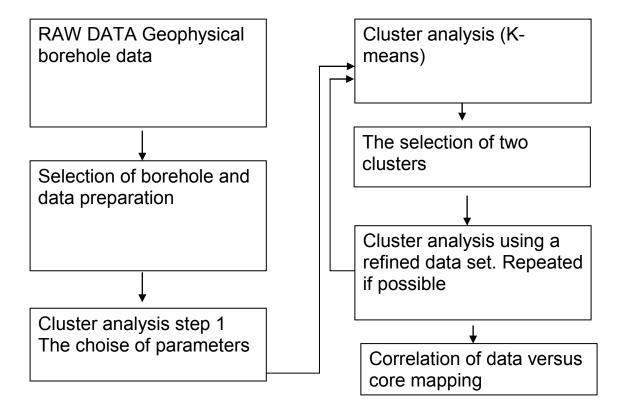
Figure 3. Established work flow schedule of the K-means cluster analysis.
