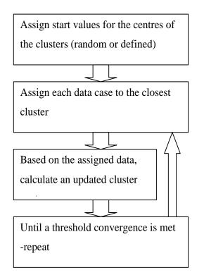
Figure. 2. An algorithm describing the K-mean Cluster analysis technique.
