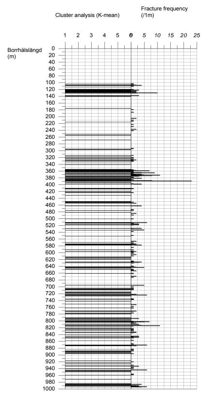
Figure 6. Results of the K-mean cluster analysis using the density, susceptibility, resistivity (140 cm and 300 cm) and the P-wave velocity parameters (based on 8020 cases). A comparison with fracture frequency data (open fractures) is by inspection yielding a certain degree of correlation.
