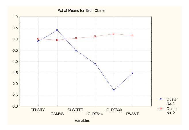
Figure 4. The Cluster K-mean analysis was performed using density, gamma, magnetic susceptibility, res140, res 300 and full-wave (P-wave). All parameters except gamma exhibit lower mean values for cluster 1 than is the case for cluster number 2. Based on this analysis, the gamma parameter was omitted and the analysis was once again performed (figure 4).
