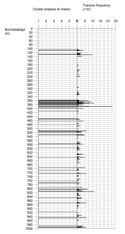
Figure 8. Result of a second K-mean cluster analysis using the density, susceptibility, resistivity (140 cm and 300 cm) and the P-wave velocity parameters (based on 757 cases). A comparison with fracture frequency data is showing good correlation.
