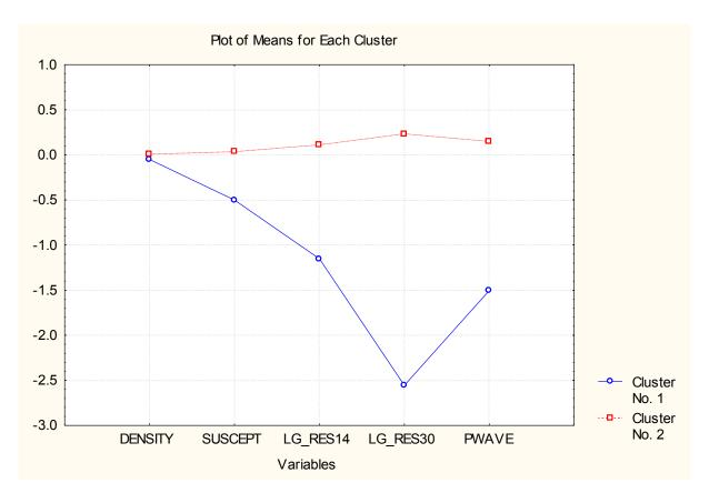
Figure 5. Result of the K-mean cluster analysis using the density, susceptibility, resistivity (140 cm and 300 cm) and the P-wave velocity parameters. The standardized mean value for cluster 1 (corresponding to fractures or fracture zones) are considerably lower for most of the geophysical parameters used in the cluster analysis than is the case for cluster 2 (corresponding to bedrock matrix).
