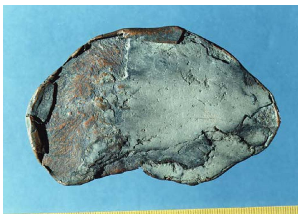
Figure 17 A 176 million years old copper (mm scale at the bottom) plate found embedded in clay in Littleham Cove, Devonshire, GB (from a presentation 2007-12-05 by L. Werme, SKB).
