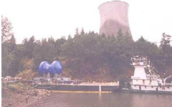
Figure 2-5 RPV Barge Transport on the Columbia River
