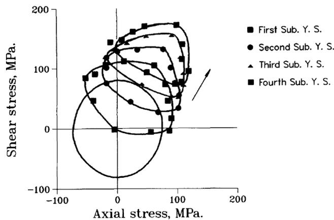
**Figure 2-3:** Subsequent yield surfaces during loading of an annealed ANSI type 304 stainless steel tubular specimen [Wu and Yeh, 1991].
