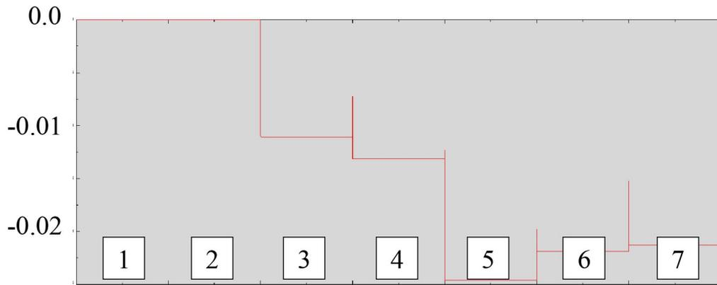
**Figure 3-7:** Plastic strain in axial direction in centre in bead 3 as a function of bead deposited. Number of bead laid is shown in white squares.
