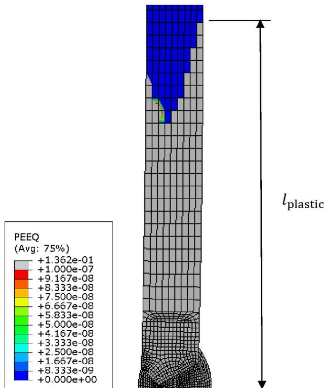
**Figure 3-1:** Equivalent plastic strain PEEQ in a pipe after a 2D welding simulation.  $l_{\text{plastic}}$  is the axial length of the pipe, measured from the centre of the X-shaped girth weld, in which plastic deformation occurs. Half of the weld is shown. Base and weld material is 316L. Mean radius of pipe  $R_m = 398$  mm. Thickness of pipe  $t = 15.9$  mm.
