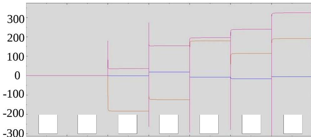
**Figure 3-6:** Radial ( $S_{11}$ , blue), axial ( $S_{22}$ , orange) and hoop ( $S_{33}$ , red) stress in centre of bead 3 as a function of bead deposited. Number of bead laid is shown in white squares. Stress is given in MPa.
