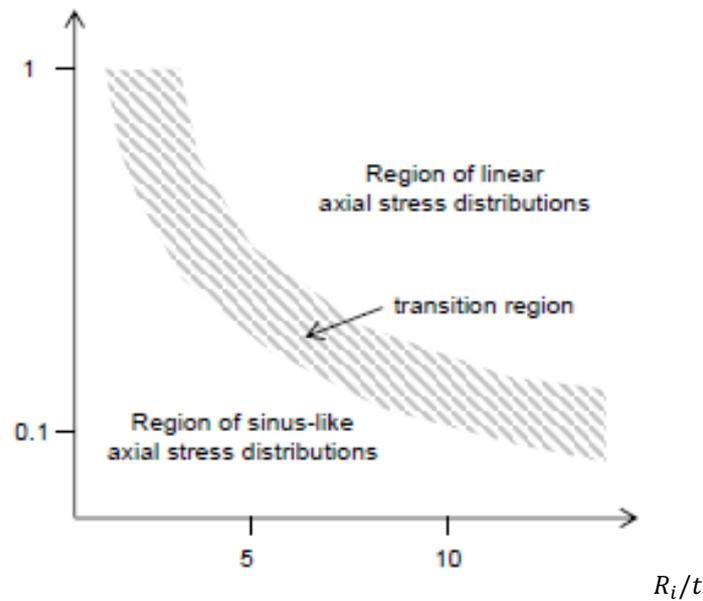
**Figure 2-2:** Sketch of regions for linear and sinusoidal stress distribution for axial stress in a pipe butt weld as a function of pipe geometry ( $R_i/t$ ) and bead size ( $b/t$ ) [Bonnaud and Gunnars, 2016a].
