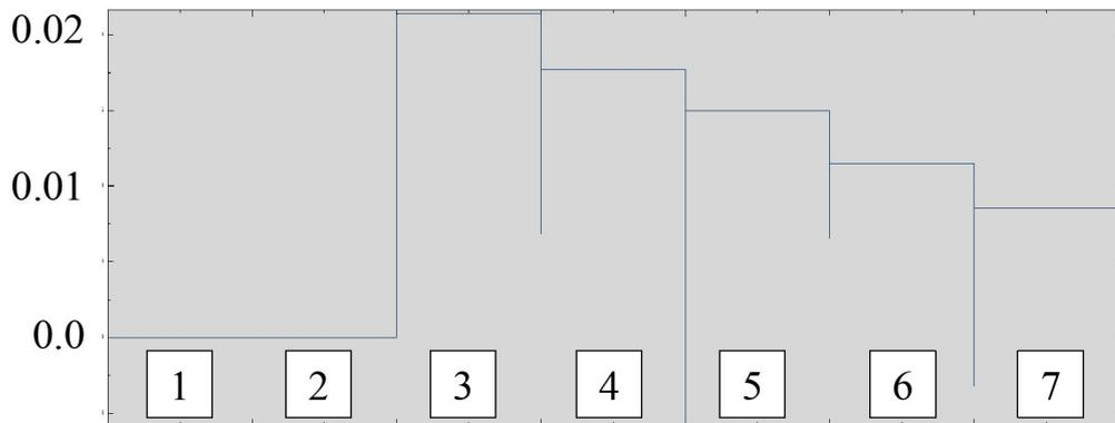
**Figure 3-8:** Plastic strain in hoop direction in centre of bead 3 as a function of bead deposited. Number of bead laid is shown in white squares.
