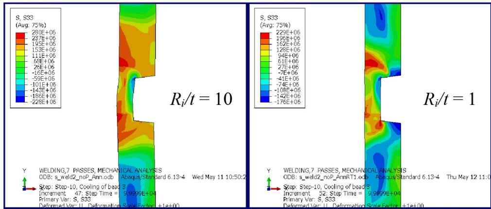
**Figure 3-13:** Hoop stress  $S_{33}$  in Pa at room temperature after bead three has been laid. Left figure:  $R_i/t = 10$ . Right figure:  $R_i/t = 1$ . Deformation scale factor is 1.
