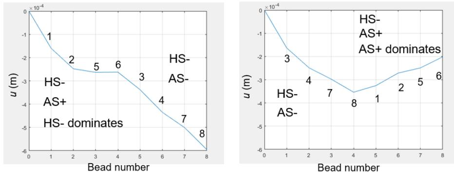
**Figure 3-4:** Radial displacement of inner surface of pipe at a double V weld as a function of bead sequence. Left figure shows radial displacement for bead sequence 1-2-5-6-3-4-7-8. Right figure shows radial displacement for bead sequence 3-4-7-8-1-2-5-6.
