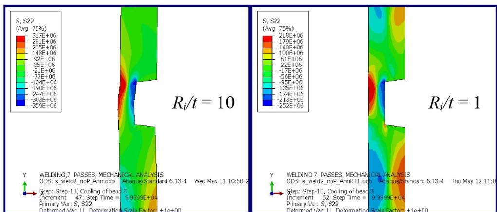
Figure 3-12: Axial stress  $S_{22}$  in Pa at room temperature after bead three has been laid. Left figure:  $R_i/t = 10$ . Right figure:  $R_i/t = 1$ . Deformation scale factor is 1.
