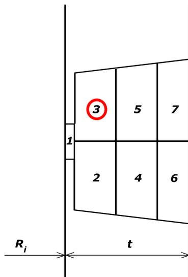
**Figure 3-5:** U-shaped girth weld with bead sequence 1 to 7. Stress and strain evolution in the centre of bead 3 is investigated.
