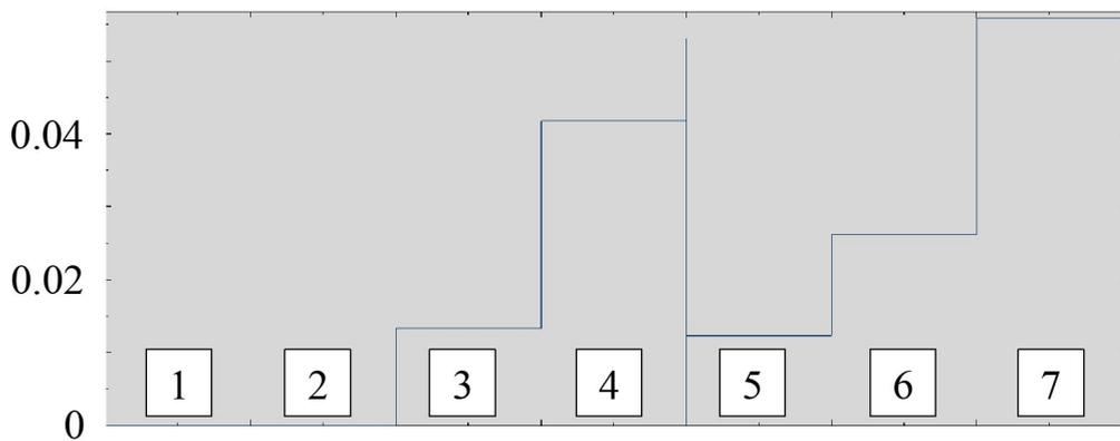
**Figure 3-9:** Equivalent plastic strain in centre of bead 3 as a function of bead deposited. Number of bead laid is shown in white squares.
