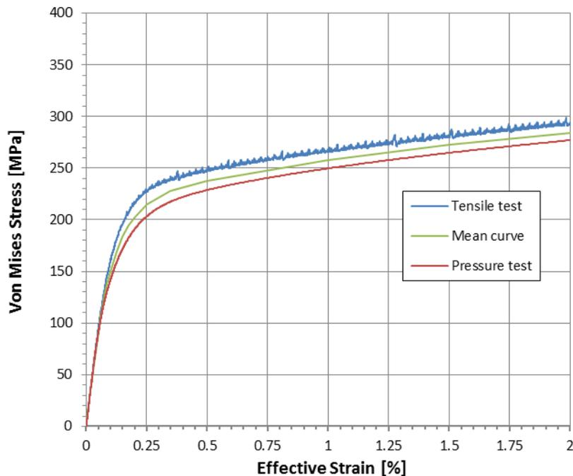
**Figure 2-4:** Experimental stress-strain curves from testing of a 316L pipe [Möller et al., 2015]. The uniaxial tensile test is conducted in the axial direction of pipe. In the multiaxial pressure test  $\sigma_{hoop} \approx 2\sigma_{ax}$ ,
