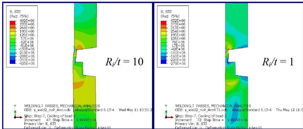
Figure 3-11: Hoop stress  $S_{33}$  in Pa at room temperature after bead two has been laid. Left figure:  $R_i/t = 10$ . Right figure:  $R_i/t = 1$ . Deformation scale factor is 1.
