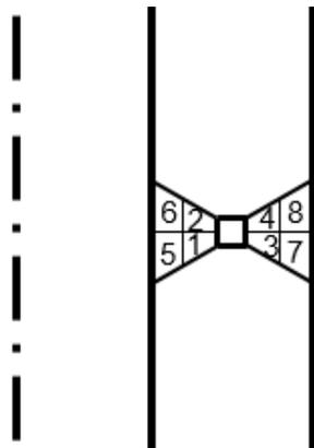
**Figure 3-2:** Weld beads defined by numbers for a double V girth weld. Wall thickness of pipe  $t = 10$  mm and inner radius  $R_i = 100$  mm.
