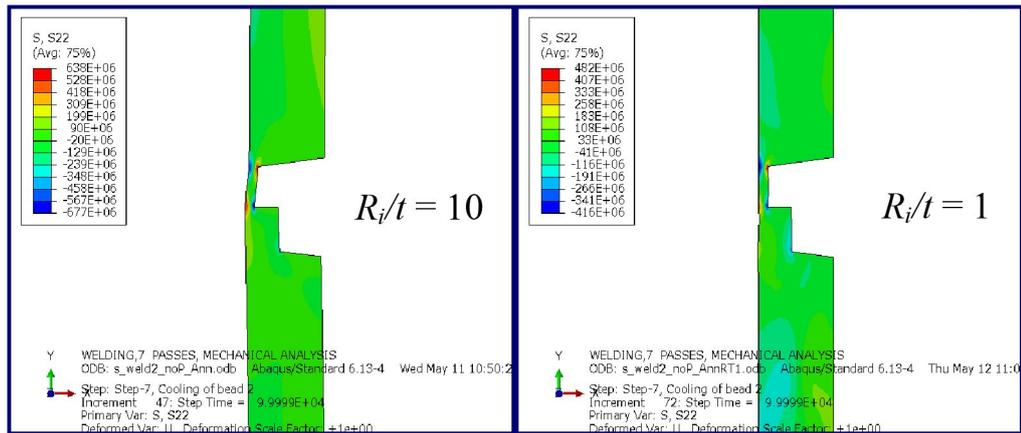
Figure 3-10: Axial stress  $S_{22}$  in Pa at room temperature after bead two has been laid. Left figure:  $R_i/t = 10$ . Right figure:  $R_i/t = 1$ . Deformation scale factor is 1.
