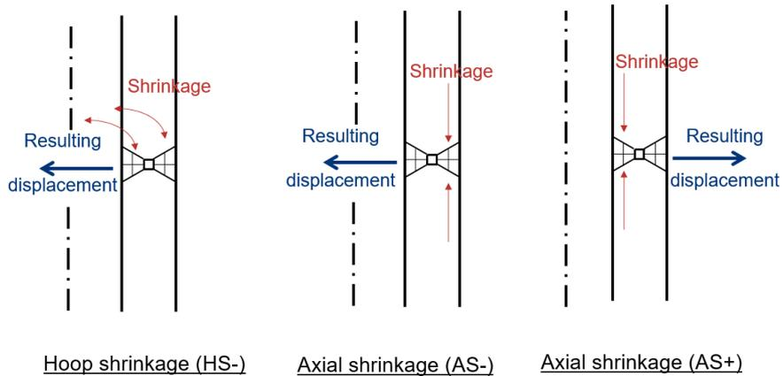
**Figure 3-3:** Resulting radial displacement as a result of hoop or axial shrinkage.
