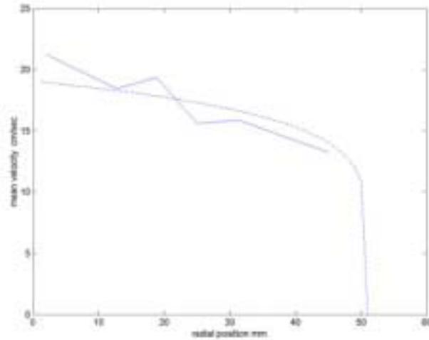
**Fig. 9.** The reconstructed radial velocity profile (broken line segments) and the theoretical velocity profile (continuous line)
