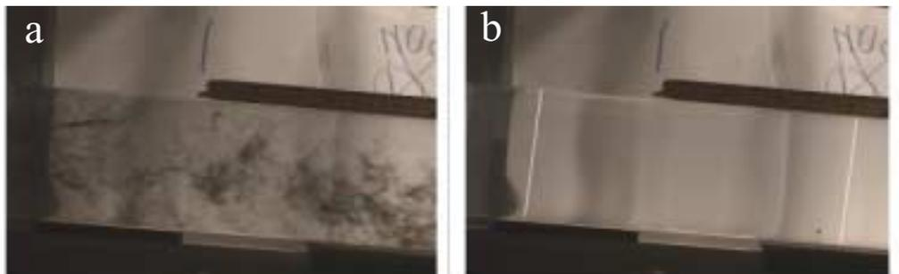
**Fig. 6.** A snapshot of the video recording showing the pipe and the colour transported from right to left (a); the position of the pixels used in the correlation analysis (b).
