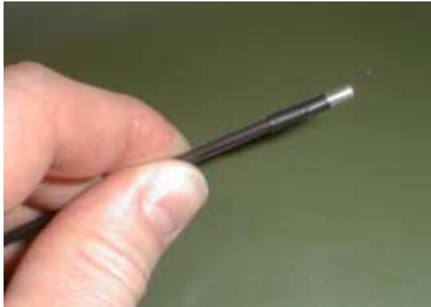
*Fig. 4. The thin scintillation detector on the tip of the light guiding fibre*
