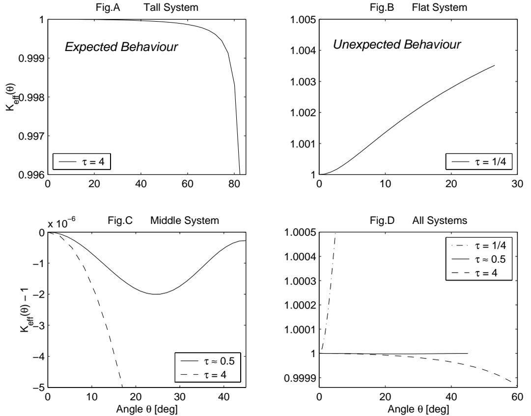
**Fig. 2.**  $k_{eff}$  dependence on the angle for tall, flat, and middle systems, Fig.C and Fig.D display the same data on different scales
