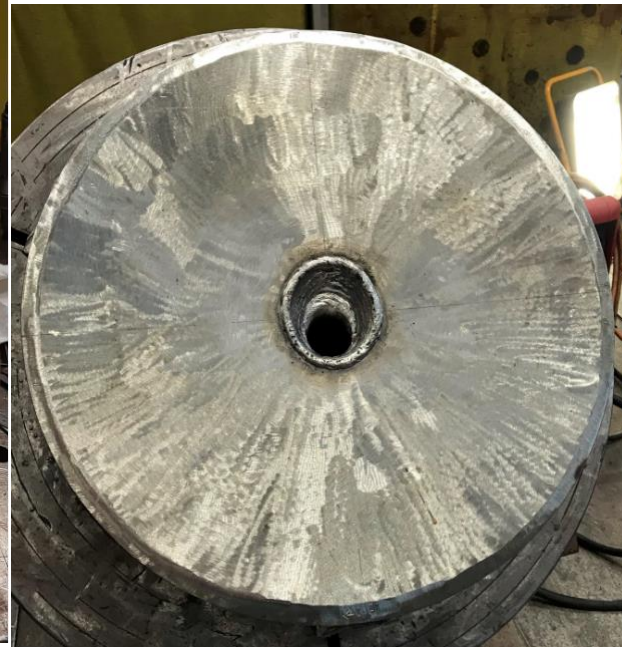
Welding the buttering
