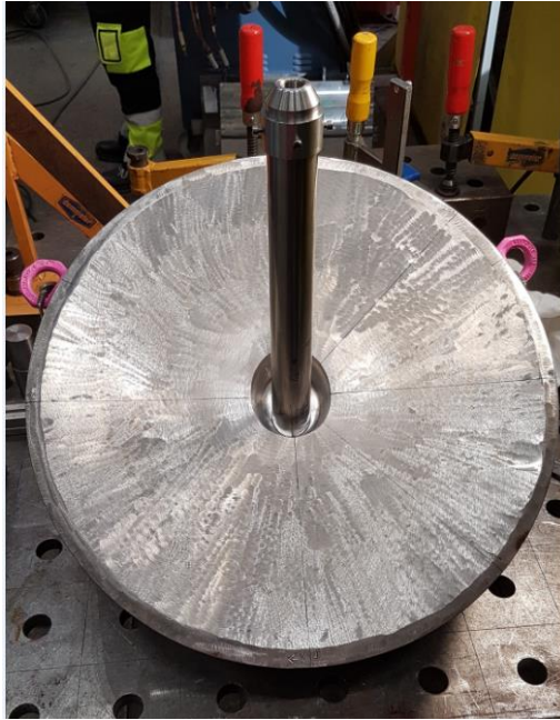
Machining the weld preparation
