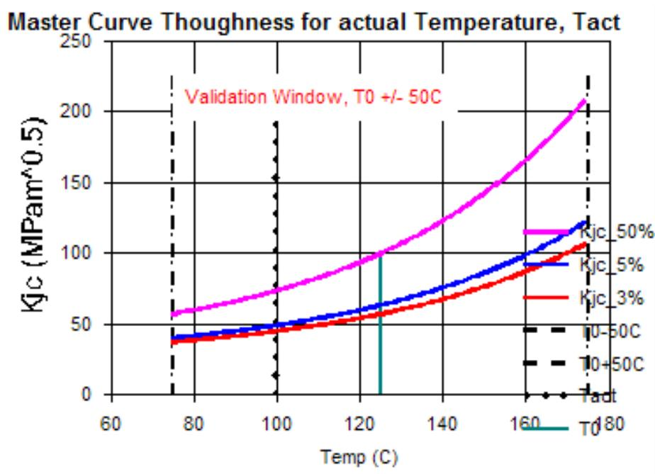
Fig. A2: ProSACC Master Curve fracture toughness evaluations of the weld based on  $T_{28J}$  value.
