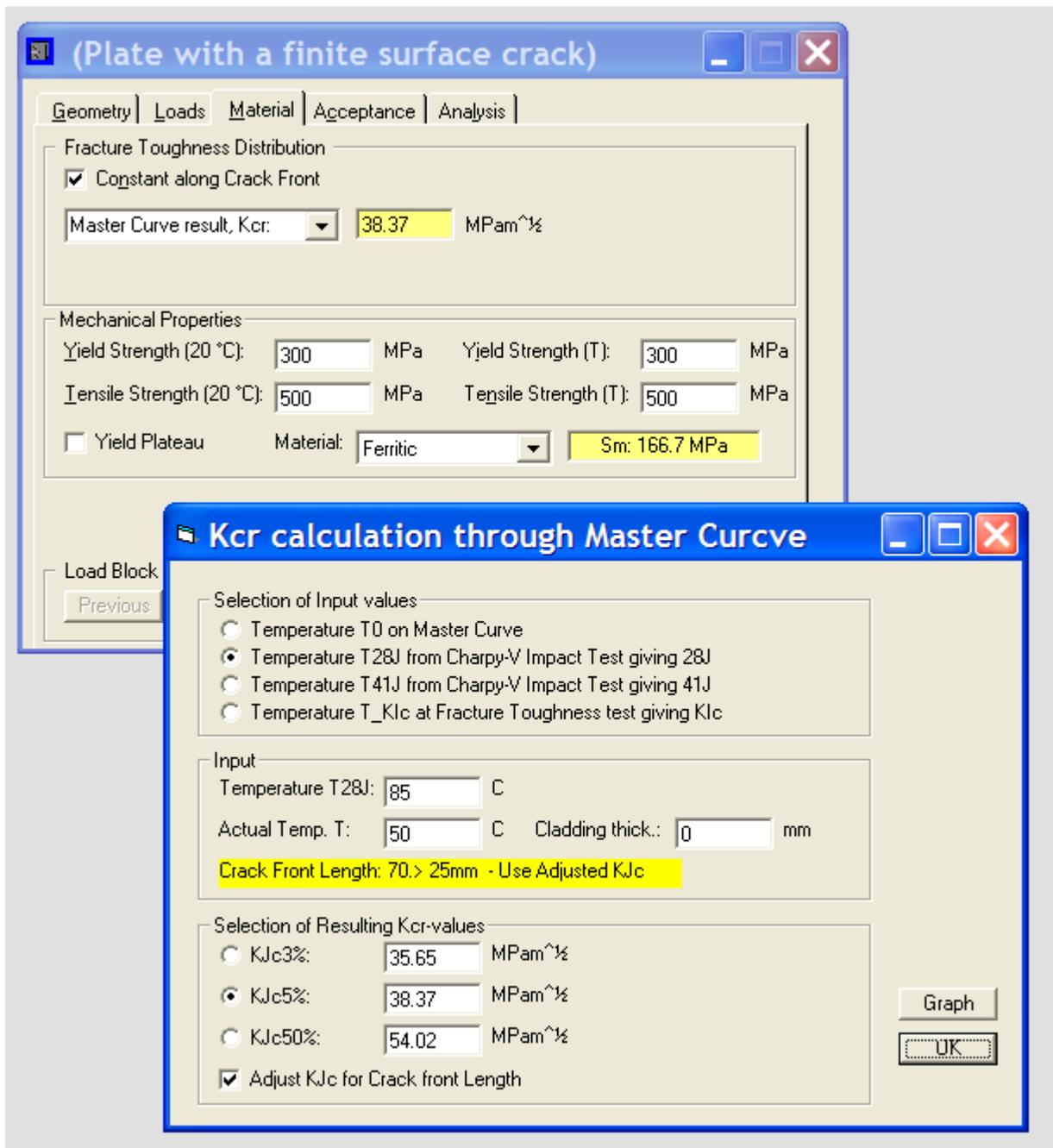
Fig. 3.5: Results of Master Curve toughness with choosing  $T_{28J}$  and 5% fracture probability and correction for 70 mm crack-front-length.
