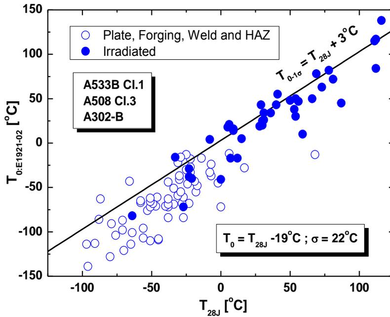
Fig. 2.4: Correlation for  $T_{28J}$  transition temperature including only western nuclear pressure vessel materials with valid  $T_0$  values.
