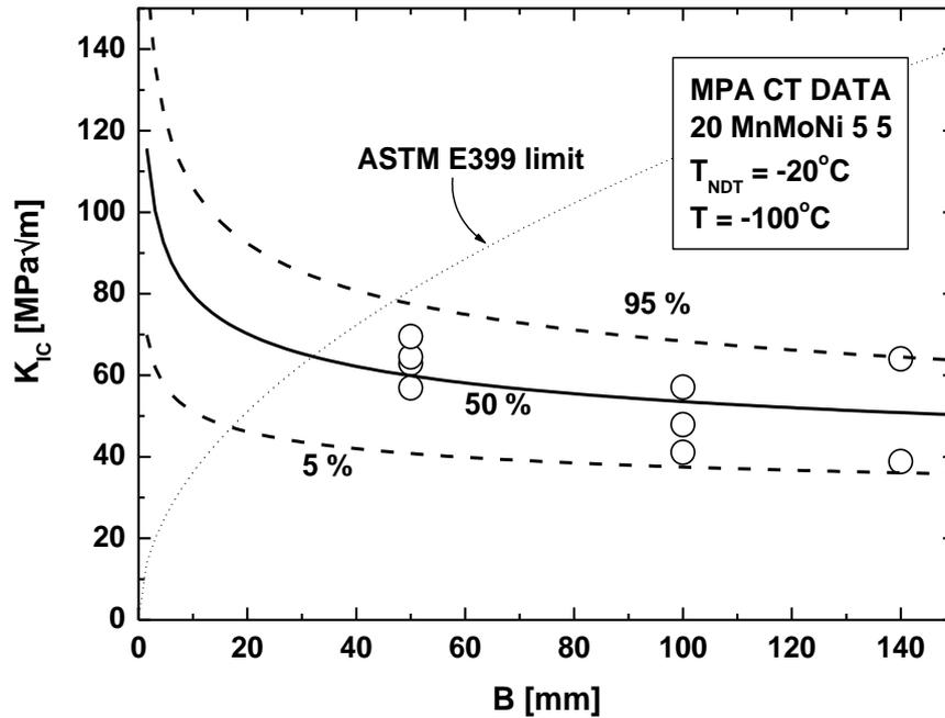
Fig. 2.3: MPA brittle fracture  $K_{Jc}$  data, for KS13, showing size effect in accordance with the Master Curve, (Issler, [1979]).
