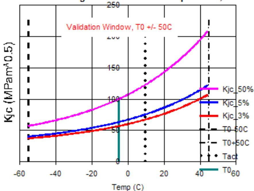
Fig. A1: ProSACC Master Curve fracture toughness evaluations of the steel based on  $T_0$  value.
