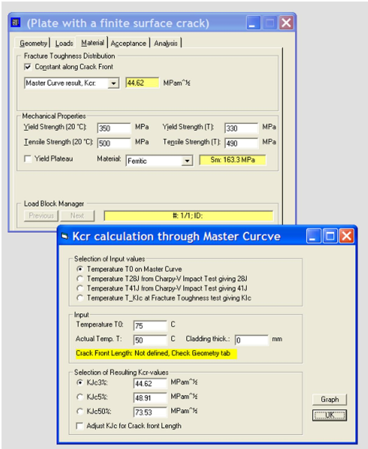
Fig. 3.2: Material box, results of Master Curve toughness for 3% fracture probability.
