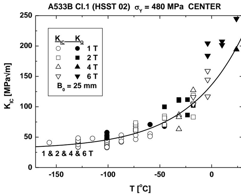
Fig. 2.2: Master Curve evaluation of brittle fracture  $K_{IC}$  data for the HSST 02 plate.
