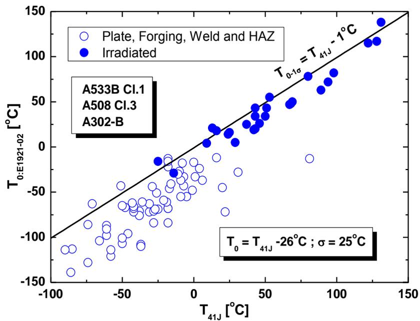
Fig. 2.5: Correlation for  $T_{41J}$  transition temperature, where only western nuclear pressure vessel materials with valid  $T_0$  values are included.
