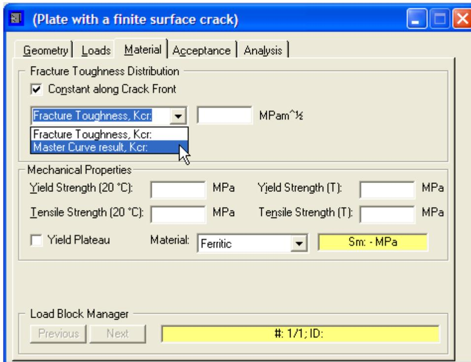
Fig. 3.1: Material box in ProSACC for input data related to fracture toughness.
