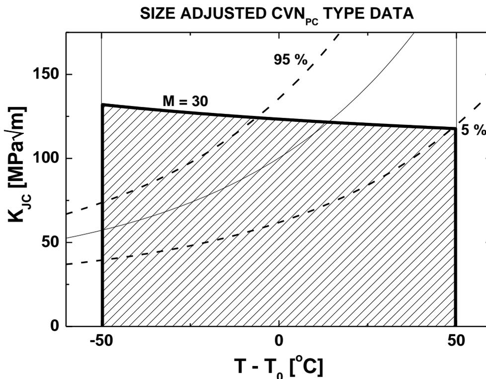
Fig. 2.6: Validation window in application of the Master Curves for the ferritic materials.
