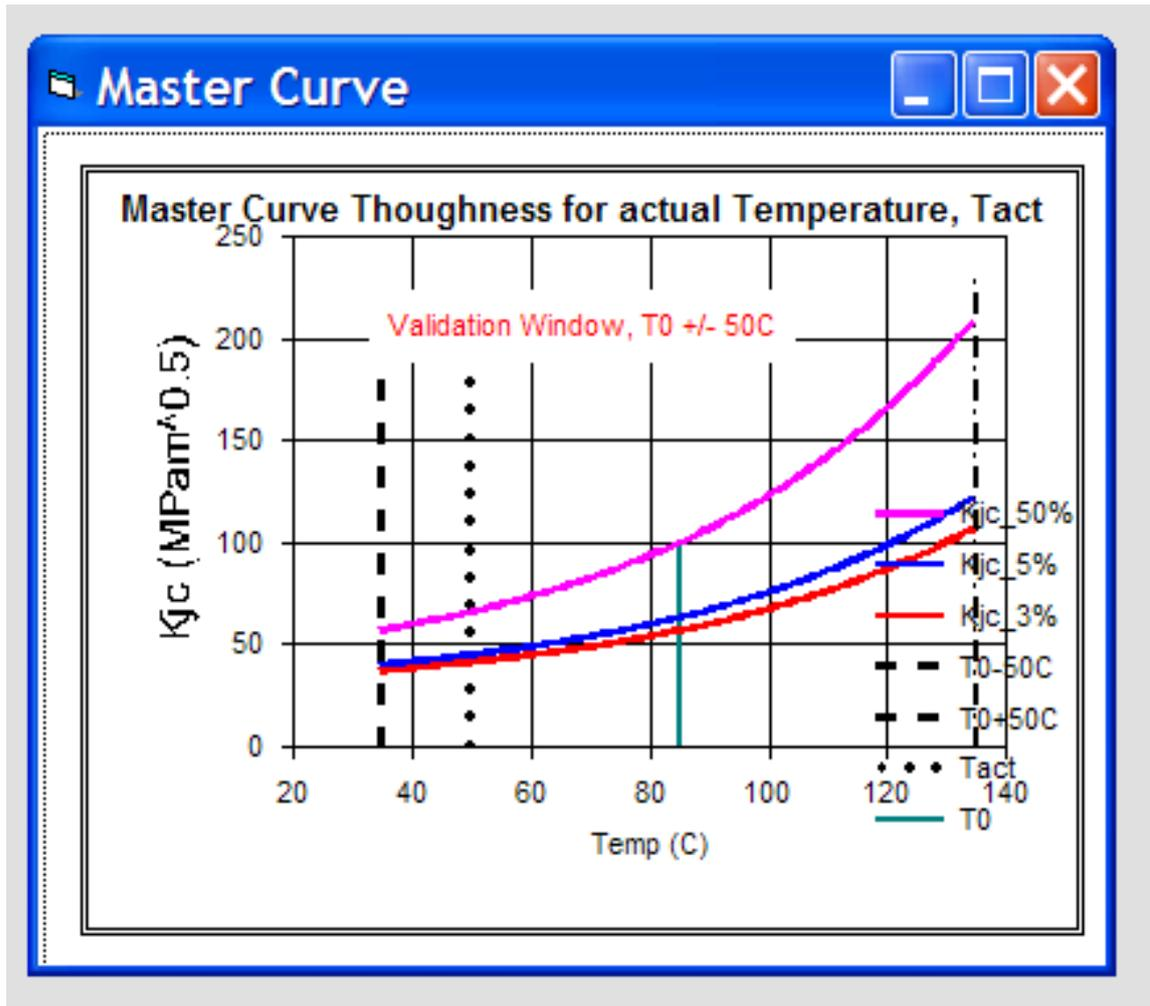
Fig. 3.4: Evaluated results in an Application window of Master Curve toughness.
