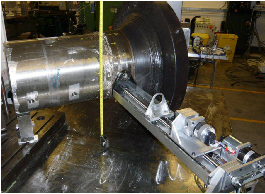
Figure 3-10 Component configuration and measurement location for the second series of DHD and iDHD measurements in the Dissimilar Metal Weld, following addition of the SS pipe weld.
