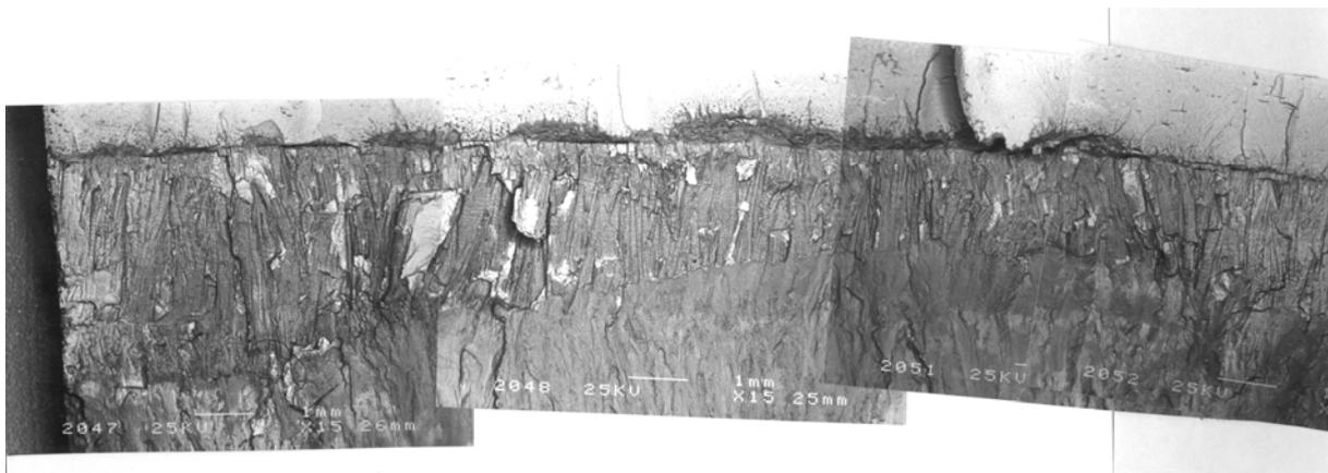
**Figure 26:** Back scatter electron SEM macrograph of specimen 301, with fatigue pre-crack tip in Inconel 182 weld metal. ID SCC and thumb-nail-shaped crack extension to weld HAZ of RPV steel can be clearly seen [3].
