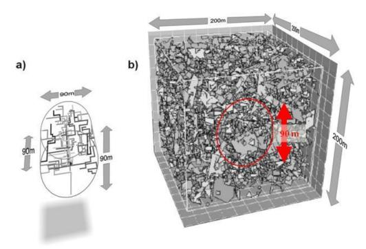
**Figure 5.** Comparison of a) a sparse channel network representing groundwater flow at the Stripa URL and b) a DFN model of "background fractures" at the TRU Block tracer experiment at Äspö (Black et al., 2013). Note that both images are at the same scale.
