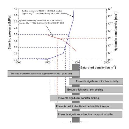
**Figure 8.** Diagram illustrating the effects of saturated density on the swelling pressure, hydraulic conductivity, and related safety functions of the buffer in a KBS-3 repository (Posiva, 2010).
