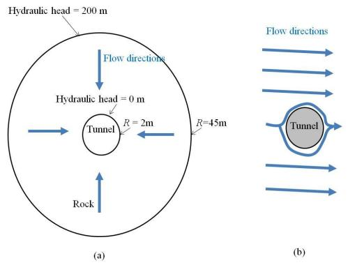
**Figure 6.** (a) Illustration of the boundary conditions and the modeling system in radial direction of the Sparse Channel Network model by Black et al (2006; 2007; and 2013) that deals with an open tunnel. *R* are the radii of inner and outer boundaries. (b) In contrast, the repository tunnel after resaturation is a no-flow boundary.
