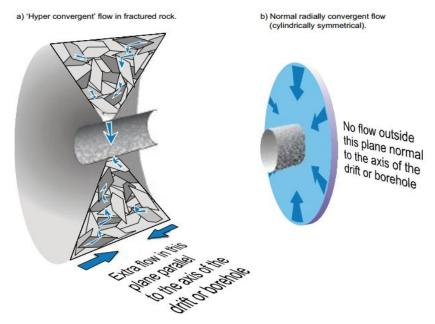
**Figure 4.** Comparison of (a) three-dimensional flow with hyper-convergence and (b) onedimensional radial flow (Black et al., 2006).
