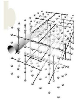
**Figure 2.** An example of Sparse Channel Network generated by 3D lattice network model. Channels are represented by dark lines, i.e., the connected bonds at the lattice corners (Black et al., 2013).
