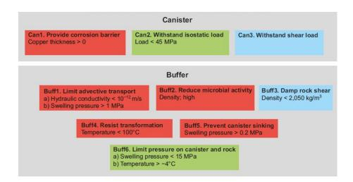
**Figure 7.** Containment related safety functions, safety function indicators, and safety function indicator criteria for the canister and buffer (based on Figure 8-2 of SKB, 2011). The colour coding relates to canister safety functions Can1 (red), Can2 (green), and Can3 (blue).
