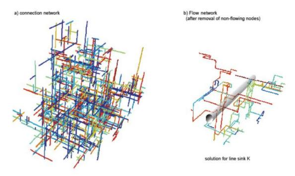
**Figure 3.** Example of how a sparse network of connections, shown in (a) is reduced to an even sparser flow network shown in (b). Note that the modelled system is a cylinder of 90-m diameter as the outer boundary and the drift is 4-m diameter as the inner boundary (Black et al., 2006). Different colors represent different networks.
