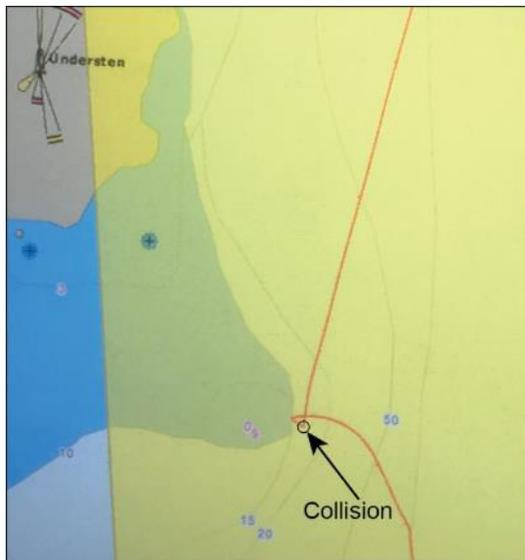
**Figure 3.** Screen dump of the ECDIS chart at the location where RV Electra hit the shoal east of Understen. Note that the actual collision occurred well outside of the 15 m depth contour. The shoal will be reported to the Swedish Maritime Administration.
