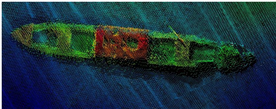
**Figure 19.** Multibeam image of ship wreck of August Thyssen at 58 m water depth. The 90 m long ship sunk in 1940 after hitting a mine. She was transporting Swedish iron ore.
