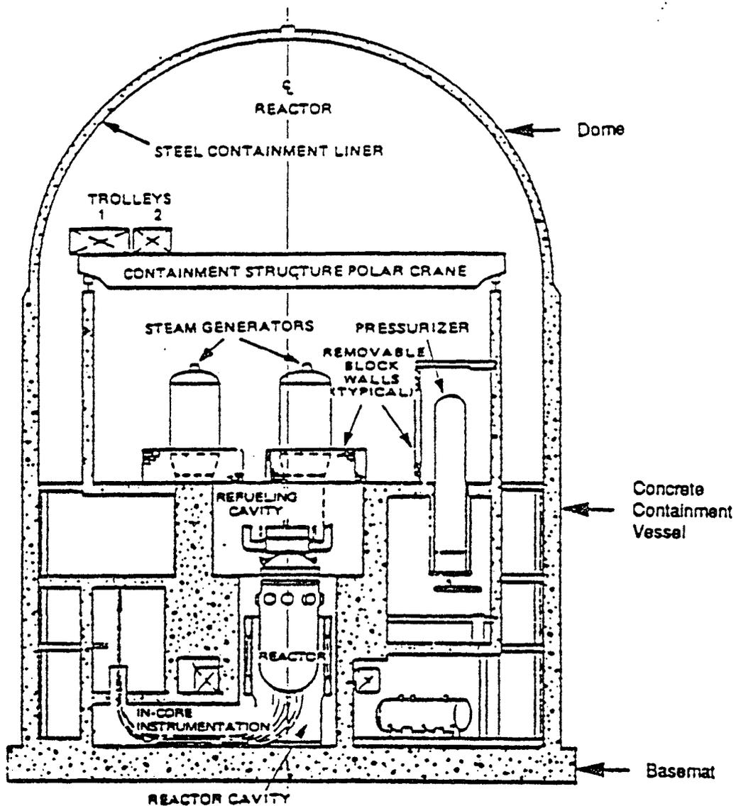
Figure 2. PWR Subatmospheric Type Reinforced Concrete Containment.
