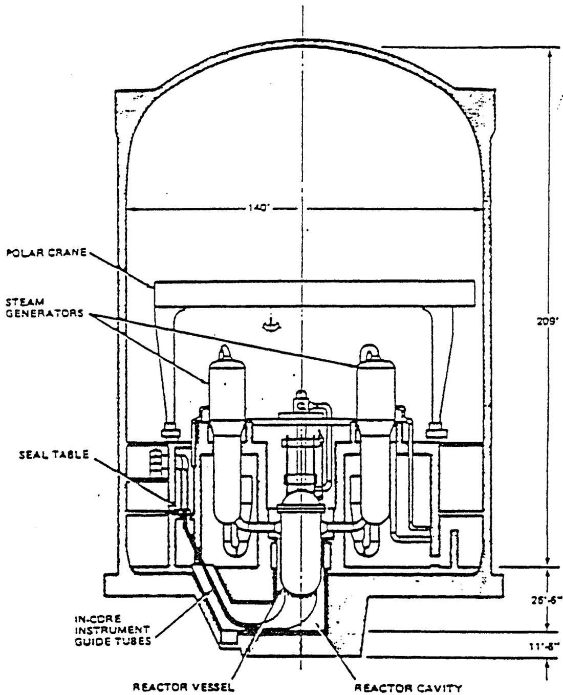
Figure 4. PWR Large/Dry Type Prestressed Concrete Containment.
