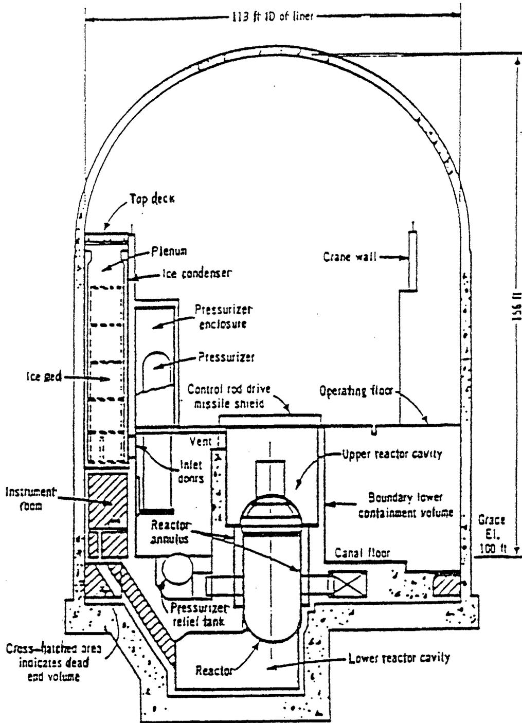
Figure 3. PWR Ice Condenser Type Reinforced Concrete Containment.
