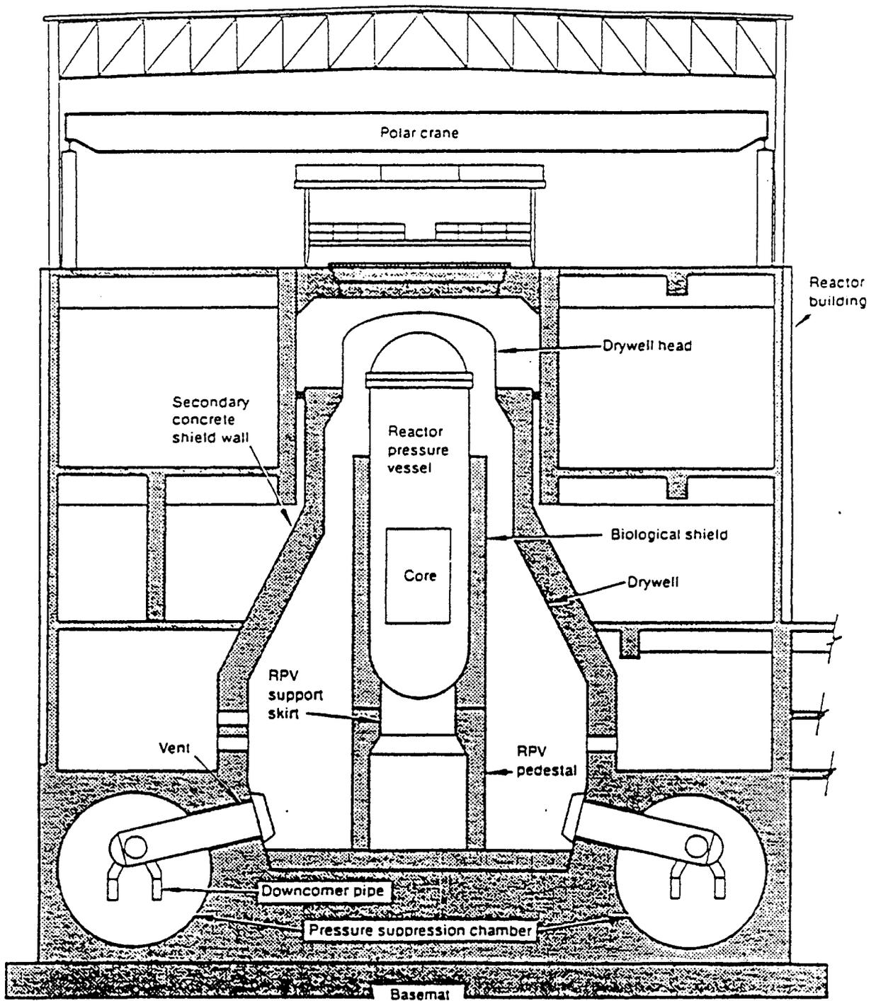
Figure 5. BWR Mark I Type Metal Containment Enclosed in a Reactor Building.
