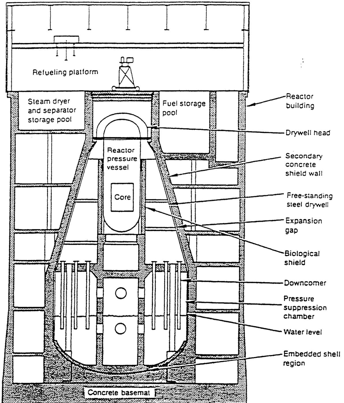
Figure 6. BWR Mark II Type Metal Containment Enclosed in a Reactor Building.
