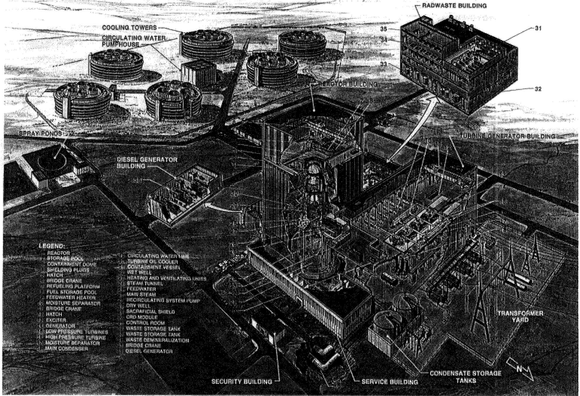
Figure 1. Cut-Away Diagram of a BWR Nuclear Power Plant Facility
