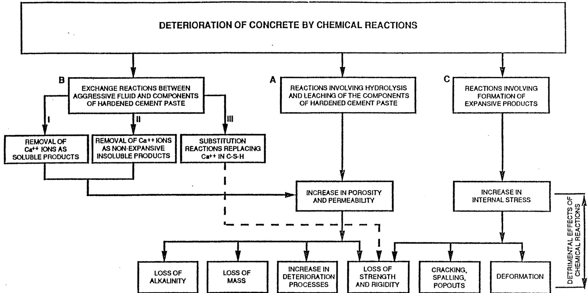
Figure 8. Types of Chemical Reactions Responsible for Concrete Deterioration. A: Softwater attack on calcium hydroxide in hydrated portland cement; B(I): Acidic solution forming soluble calcium compounds; B(II): Solutions of oxalic acids and its salts, forming calcium oxalate; B(III): Long-term seawater attack; C: Attacks of sulfate and alkali-aggregate, and corrosion of steel in concrete. Source: ORNL/NRC/LTR-90/17
