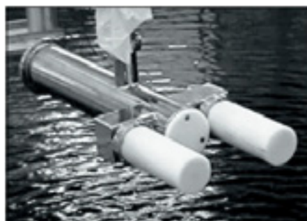
Figure 2: The Fork Detector. The prongs are placed around the fuel assembly to be measured. Image from STUK report STUK-YTO-TR 175, 2001
