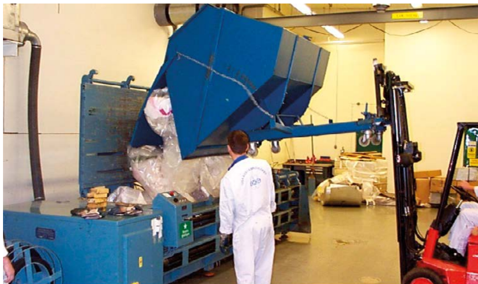
Figure A3-1. Compaction of soft LLW into square bales at Oskarshamn.
