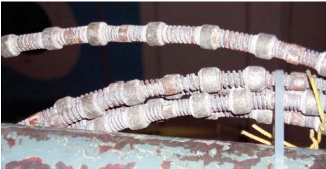
Figure 7-12. Close up of diamond wire saw blade.
