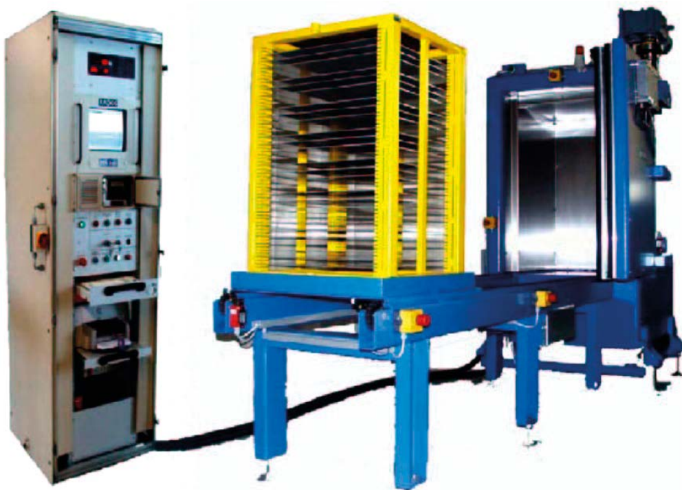
Figure A3-3. RADOS Mobile Clearance Measurement Station.
