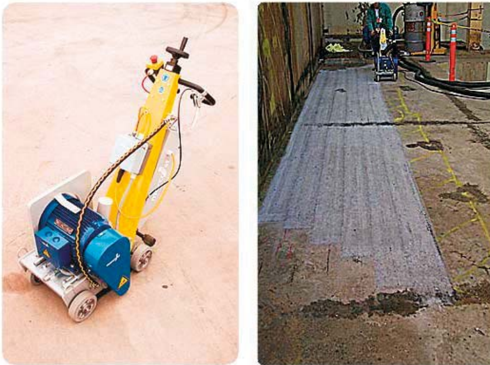
Figure 7-9. Floor Shaver and the resulting floor surface.
