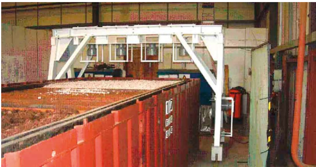
Figure A3-7. ISO Container Monitor for Bulk LLW.
