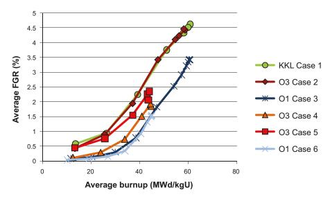
Figure 6-2. Calculated average fission gas release at the end of each cycle for the BWR cases.
