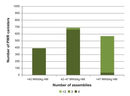
**Figure 5-3.** The PWR canisters to be deposited divided into groups with respect to the average burnup of the encapsulated assemblies. The number of assemblies in the canister is indicated by different colours. The total number of PWR canisters is 1,652.
