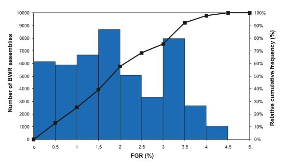
*Figure 6-4.* The number of BWR assemblies in different FGR intervals and relative cumulative frequency of FGR in BWR assemblies.
