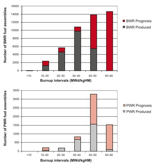
**Figure 2-1.** Burnup distribution of the spent fuel assemblies stored in Clab 31 December 2007 (grey colours) and prognosis of the burnup distribution for the assemblies resulting from the future operation of the nuclear power plants (red colours) as assumed for the reference scenario used by SKB.
