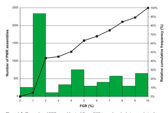
**Figure 6-5.** The number of PWR assemblies in different FGR intervals and relative cumulative frequency of FGR in PWR assemblies.
