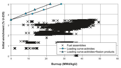
Figure 4-3. Loading curves for BWR-canisters with 12 identical fuel assemblies and enrichment and average burnup for the assemblies currently stored in Clab /SKBdoc 1193244/.
