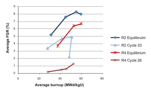
**Figure 6-3.** Calculated average fission gas release at the end of each cycle for the PWR cases. The drop in burnup and FGR for R2 (Ringhals 2) Cycle 33 is explained by that only the low burnup assemblies were loaded in the last cycle.
