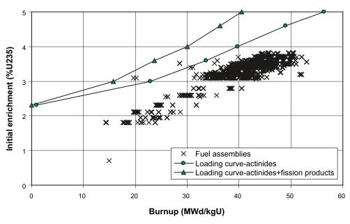
Figure 4-4. Loading curves for PWR-canisters with 4 identical fuel assemblies and enrichment and average burnup for the assemblies currently stored in Clab /SKBdoc 1193244/.
