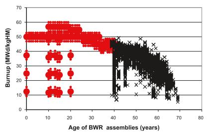
**Figure 2-3.** The burnup and age in 2045 of the BWR assemblies included in the SKB reference scenario. Assemblies that are currently stored in Clab are marked with black and assemblies from the future operation are marked with red. Large red dots represent batch average discharge burnup and small red dots represent standard deviation in burnup, i.e.  $\pm 3$  MWd/kgU, averaged over single fuel assemblies included in a batch.
