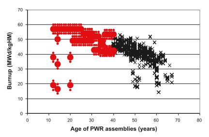
Figure 2-4. The burnup and age in 2045 of the PWR assemblies included in the reference scenario. Assemblies that are currently stored in Clab are marked with black and assemblies from the future operation are marked with red. Large red dots represent batch average discharge burnup and small red dots represent standard deviation in burnup, i.e.  $\pm 3$  MWd/kgU, averaged over single fuel assemblies included in a batch.
