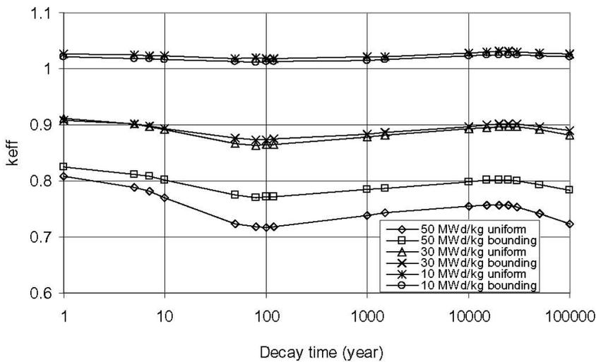
**Figure 23:** PWR  $k_{eff}$  vs. decay time for bounding and uniform axial burnup distribution, actinides and fission products (SKBdoc 1193244, Figure 38)
