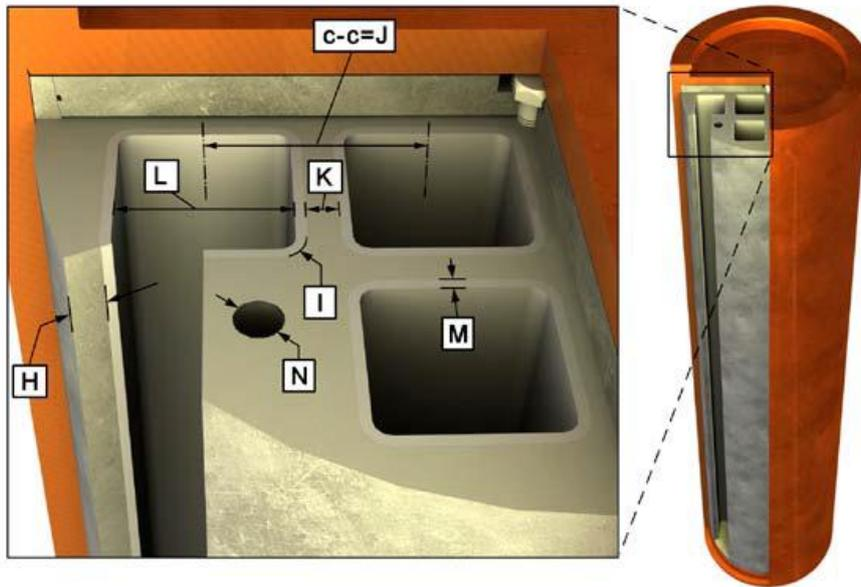
**Figure 15:** Insert (BWR) channel tubes with dimensions for PWR fuel, see Table 18 (SKB TR-10-14, Figure 3-5)
