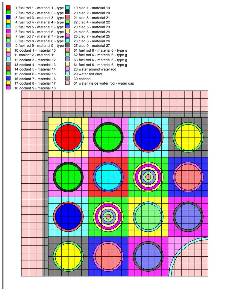
Figure A.2: NEWT geometry for OECD Phase IIIB benchmark
