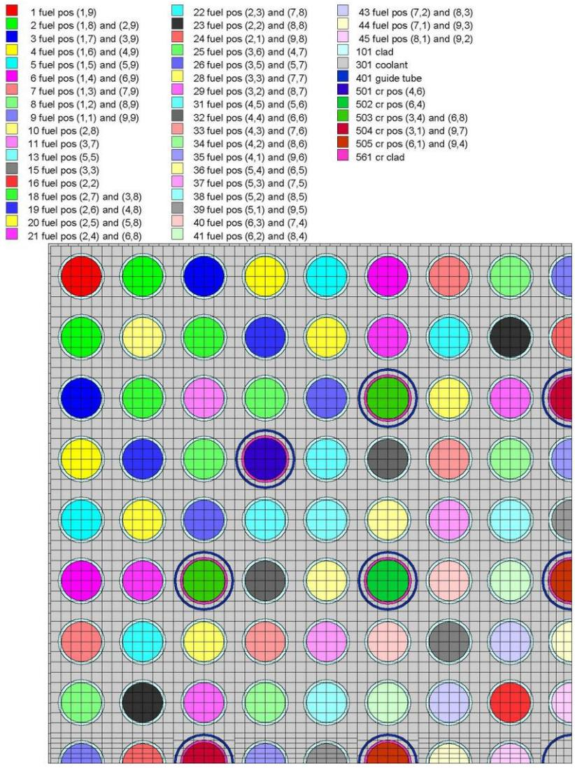
Figure A.7: Phase IID case 4 geometry model for NEWT
