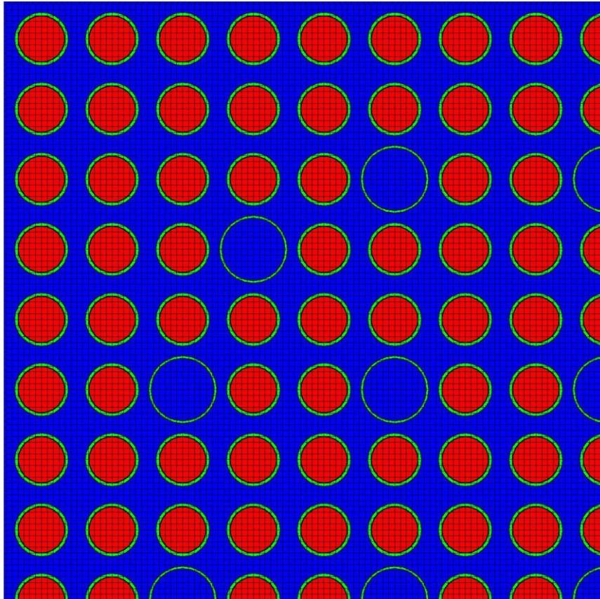
**Figure 27:** NEWT PWR fuel assembly lattice (1/4 symmetry)
