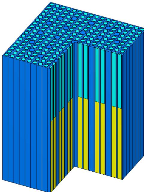
**Figure 26:** KENO V.a PWR fuel assembly lower end model (front right quarter cut away)
