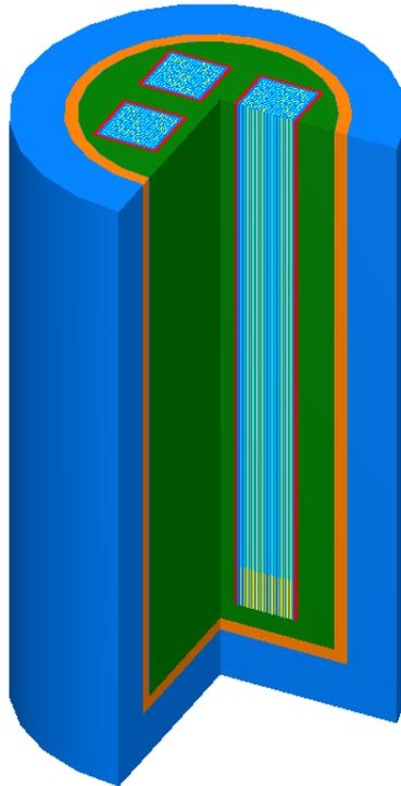
**Figure 28:** KENO V.a PWR fuel canister (top 1/2 and front right 1/4 plus a bit more cut away) with fuel
