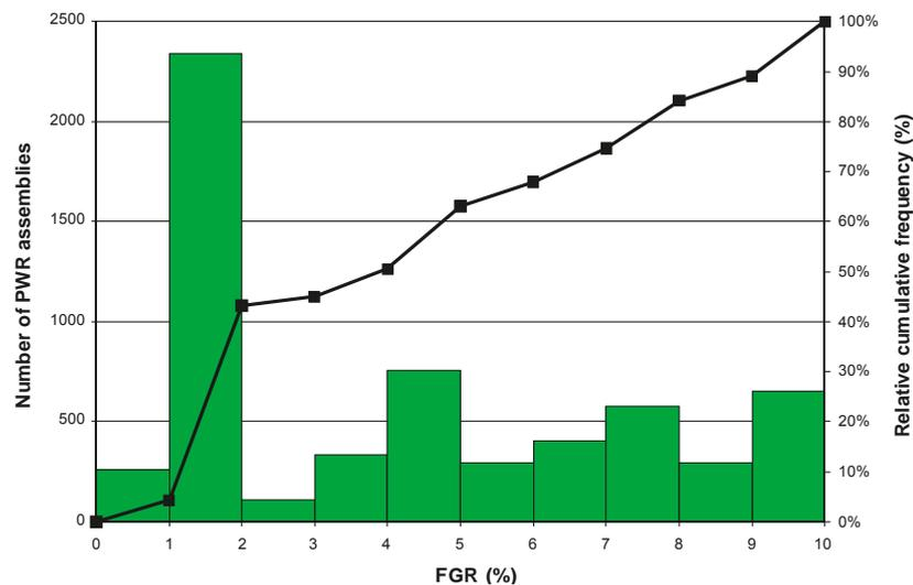
**Figure 8:** PWR assemblies in FGR intervals and FGR relative cumulative frequency (SKB TR-10-13, Figure 6-5)
