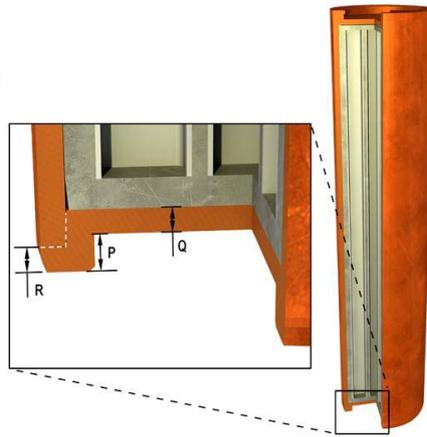
**Figure 13:** Copper base dimensions, see Table 17
