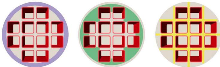
**Figure 18:** “Testing areas for BWR insert. The areas investigated with the various methods are angle scanning (lilac), normal scanning (green) and transmission testing (yellow)”
