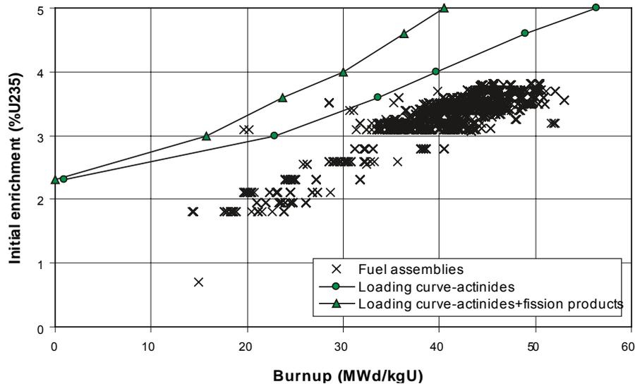
**Figure 4:** Loading curves for PWR-canisters for assemblies currently stored in Clab (SKB TR-10-13, Figure 4-4).
