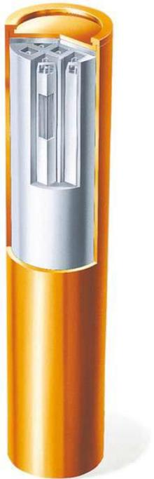
**Figure 10:** Reference canister (BWR fuel)
