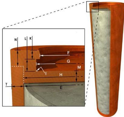
**Figure 12:** Copper lid dim., see Table 17
