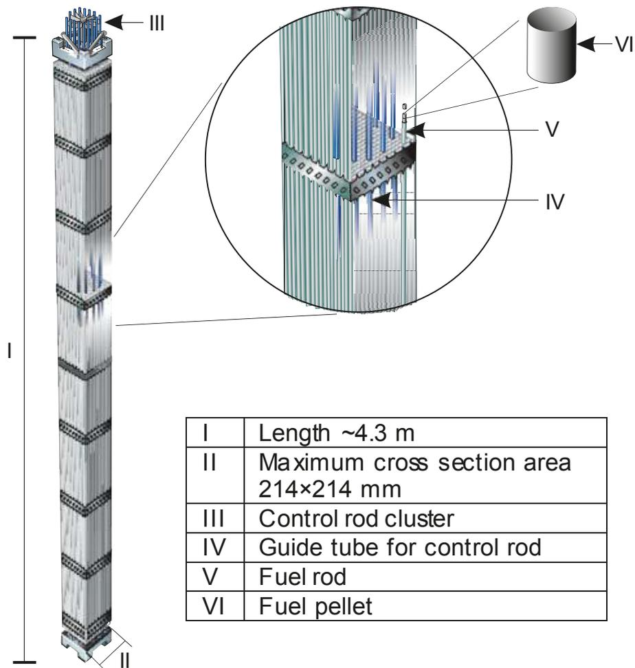
**Figure 1:** A PWR fuel assembly. (SKB TR-10-13, Figure 2-5)
