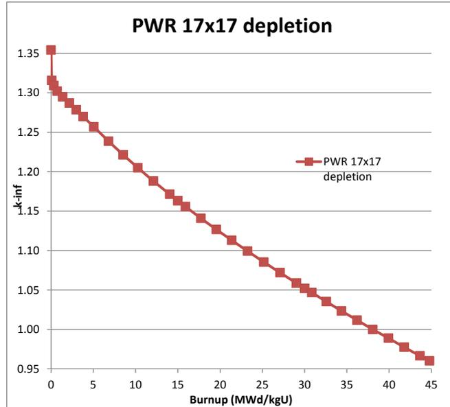
**Figure 29:** PWR 17x17 assembly depletion  $k_{inf}$  under hot full power reactor conditions
