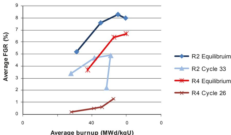
**Figure 7:** “Calculated average fission gas release at the end of each cycle for PWR cases” (SKB TR-10-13, Figure 6-3).
