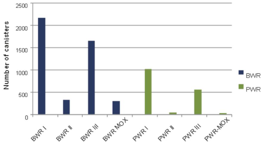
**Figure 6:** BWR and PWR canister inventory per canister type (SKB TR-10-13, Figure 6-1)
