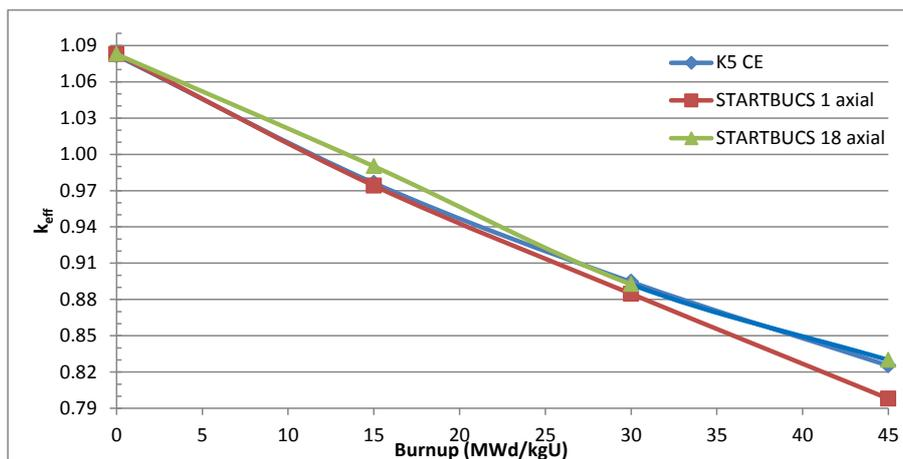
**Figure 30:** Calculation results for PWR fuel canister using different methods and models
