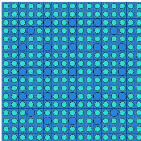
**Figure 25:** KENO V.a PWR fuel assembly lattice
