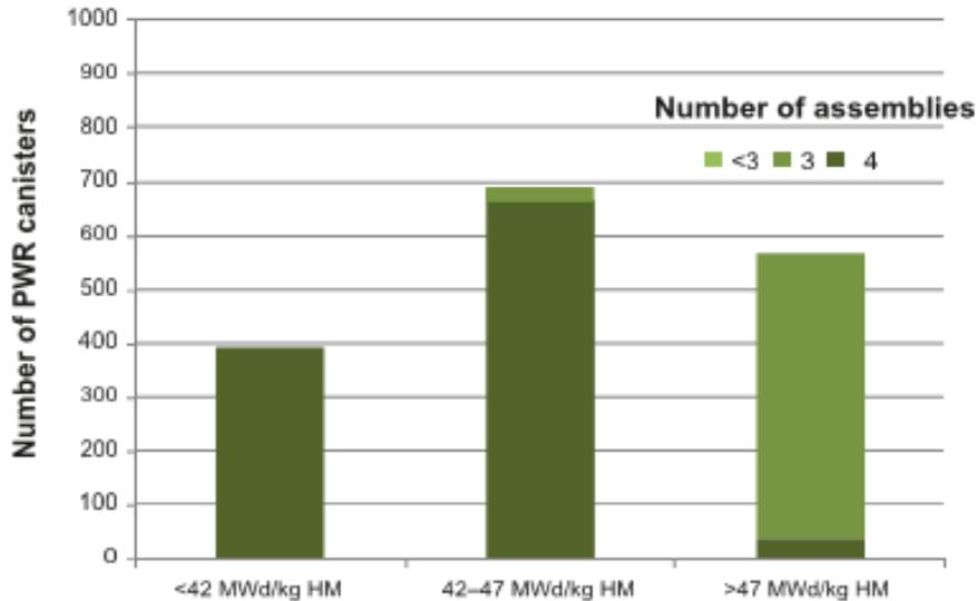
Figure 5: PWR canisters in groups with average burnup and assemblies per canister shown (SKB TR-10-13, Figure 5-3).
