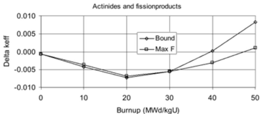
**Figure 21:** The end effect as function of burnup for different axial burnup distribution for PWR (SKBdoc 1193244, Figure 20)
