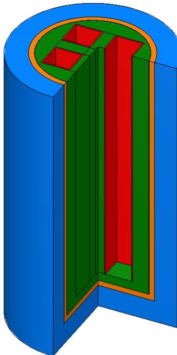
**Figure 24:** KENO V.a PWR fuel canister (top half and front right 1/4 plus a bit more cut away) without fuel
