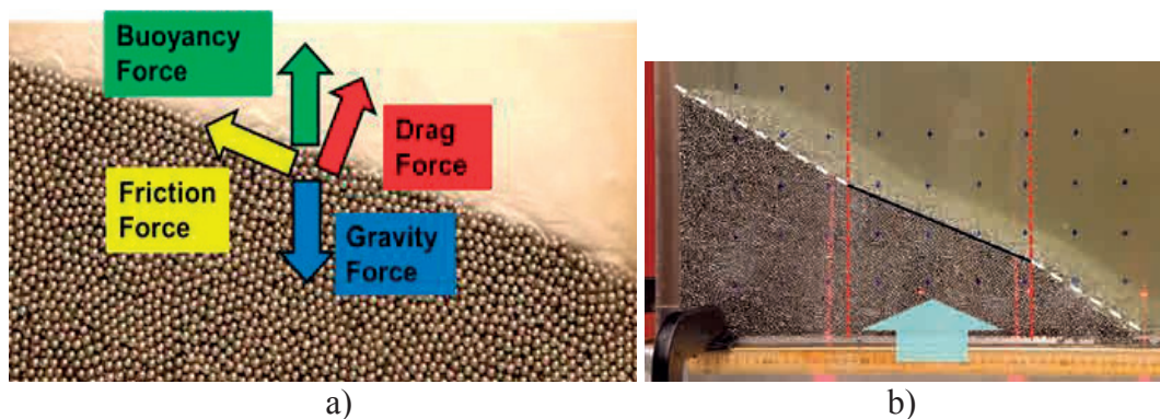
Figure 3.46. (a) Schematic of the forces acting on particles near the top bed surface; (b) shape of the bed when gas is injected only under one section of the bed.
