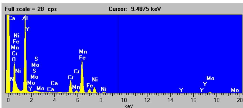
Fig. 9 EDS spectrum from an Al-rich inclusion in material C.
