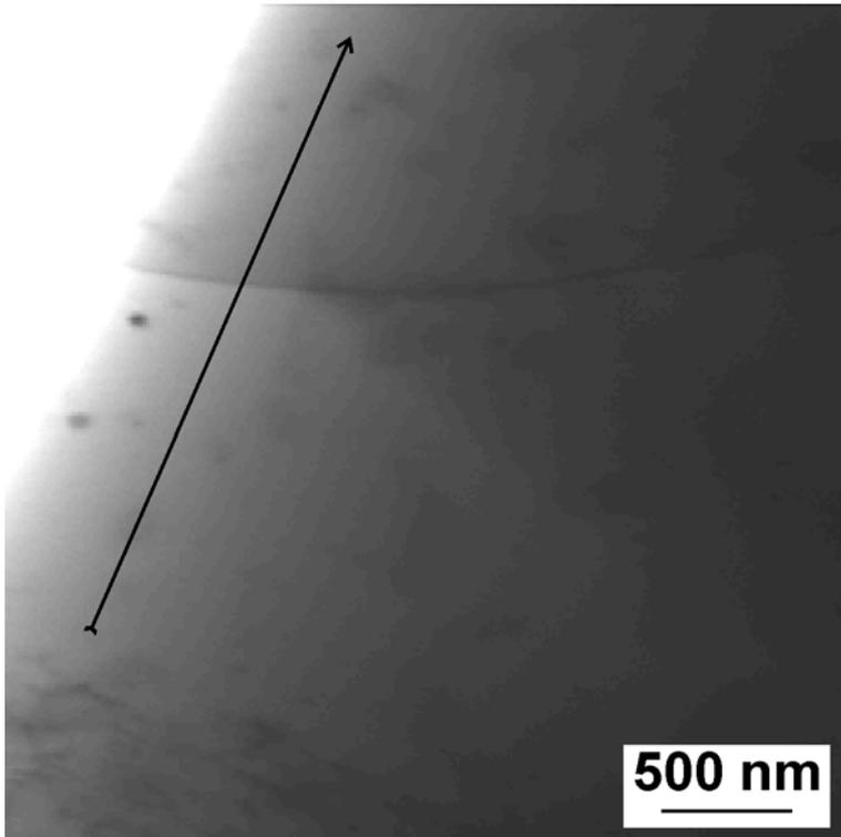
Fig. 2 STEM image, showing a grain boundary in material A. The arrow shows the EDS profile.
