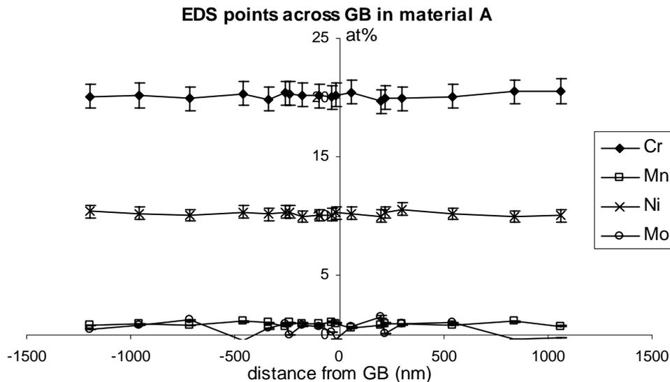
Fig. 1 STEM-EDS measurements across a grain boundary in material A. The effective spot size was approximately 2 nm. Close to the grain boundary, the step size was around 20 nm.
