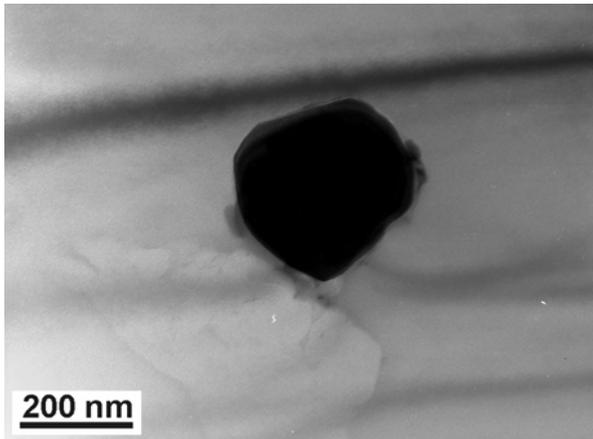
Fig. 7 Bright-field image of an Y-rich inclusion in material C.
