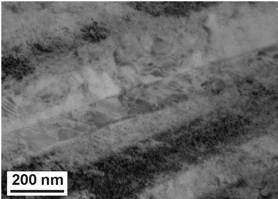
Fig. 5 Twin laths in the low N material after cold deformation (B).
