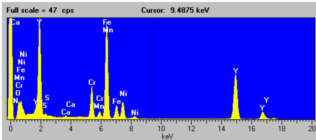
Fig. 8 EDS spectrum from an Y-rich inclusion in material C.
