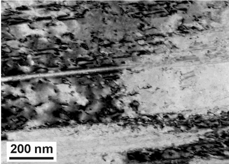
Fig. 6 Twin laths in the high N material after cold deformation (D).
