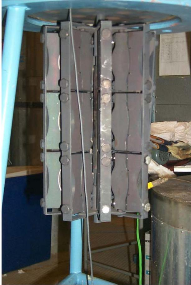
*Figure 5: Set-up of CBB test specimen holders in the autoclave.*
