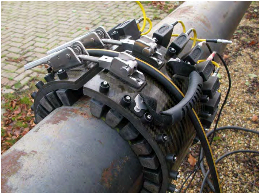
Figure 3.14: Example of a transducer collar from Plant Integrity Ltd.
