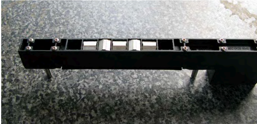
Figure 3.13: Example of a transducer section from Plant Integrity Ltd.
