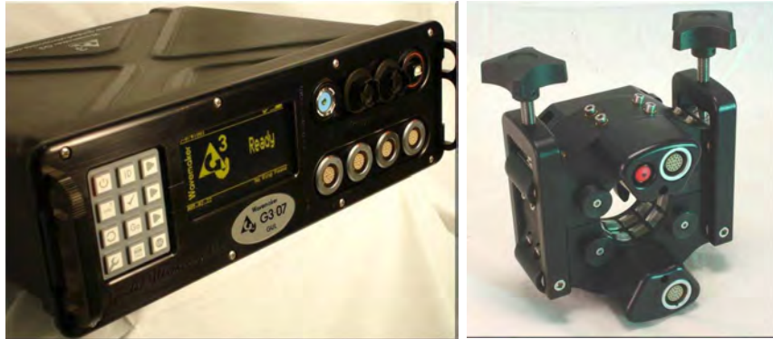
Figure 3.3: The Wavemaker instrument from Guided Ultrasonics Ltd. (left) and multiple transducer ring (right).
