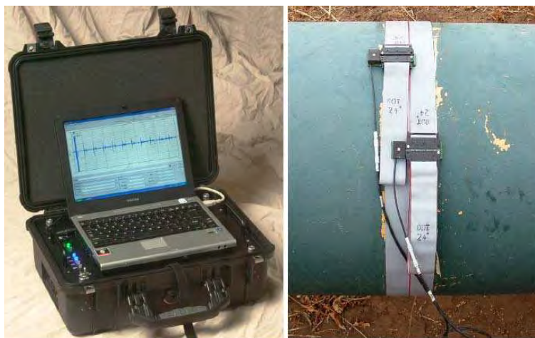
Figure 3.6: The MsSR3030 instrument from Guided NDE LLC, USA.
