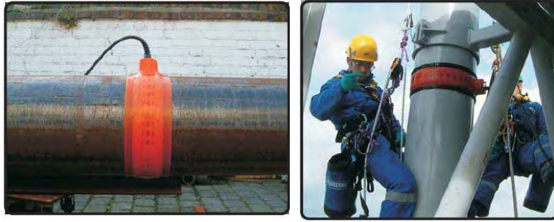
Figure 3.18: Encapsulated transducers used in PIMS.
