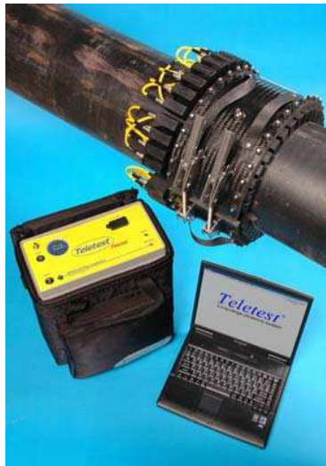
Figure 3.4: The Teletest instrument from Plant Integrity Ltd.
