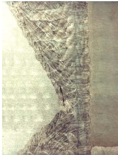
Figure 54 Etched steam generator weld. The section through the component shows the weld (and pipe's) radial/axial section. The surface from which probes could be scanned is the pipe external surface which is located at the top of the figure. Defects of general concern for the inspection are stress corrosion cracking initiating on the internal pipe surface which is located at the bottom of the figure
