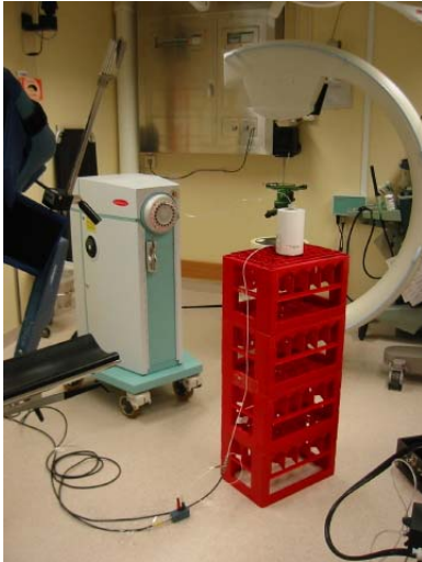
Figure 3 The SSI well-type ion chamber on top of the low-scattering plastic boxes used to position the centre of the chamber at 1 meter above the floor.
