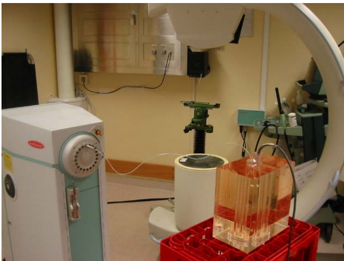
Figure 4 The Farmer-in-Phantom system used as an on-site constancy control of the well-type chamber. The plastic source-channel used to guide the source from the afterloading equipment to the irradiation position is also seen.
