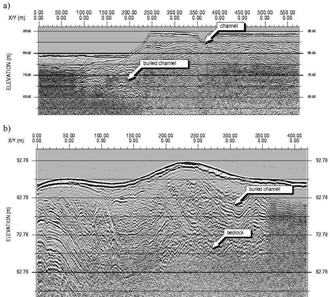
Figure 18. GPR profiles measured at the delta east of the Moredalen kursu-valley (location of profiles is given in Figure 16): a. Profile I is measured south-westward from the plainland up onto the delta, turns north-westward across a former channel and turns back north-eastward to the front of the delta, a U-turn, and b. Profile III is measured from south and northward across the Moreån brook, across a eastern wedge of the delta and thereafter out on the plainland north of the delta.
