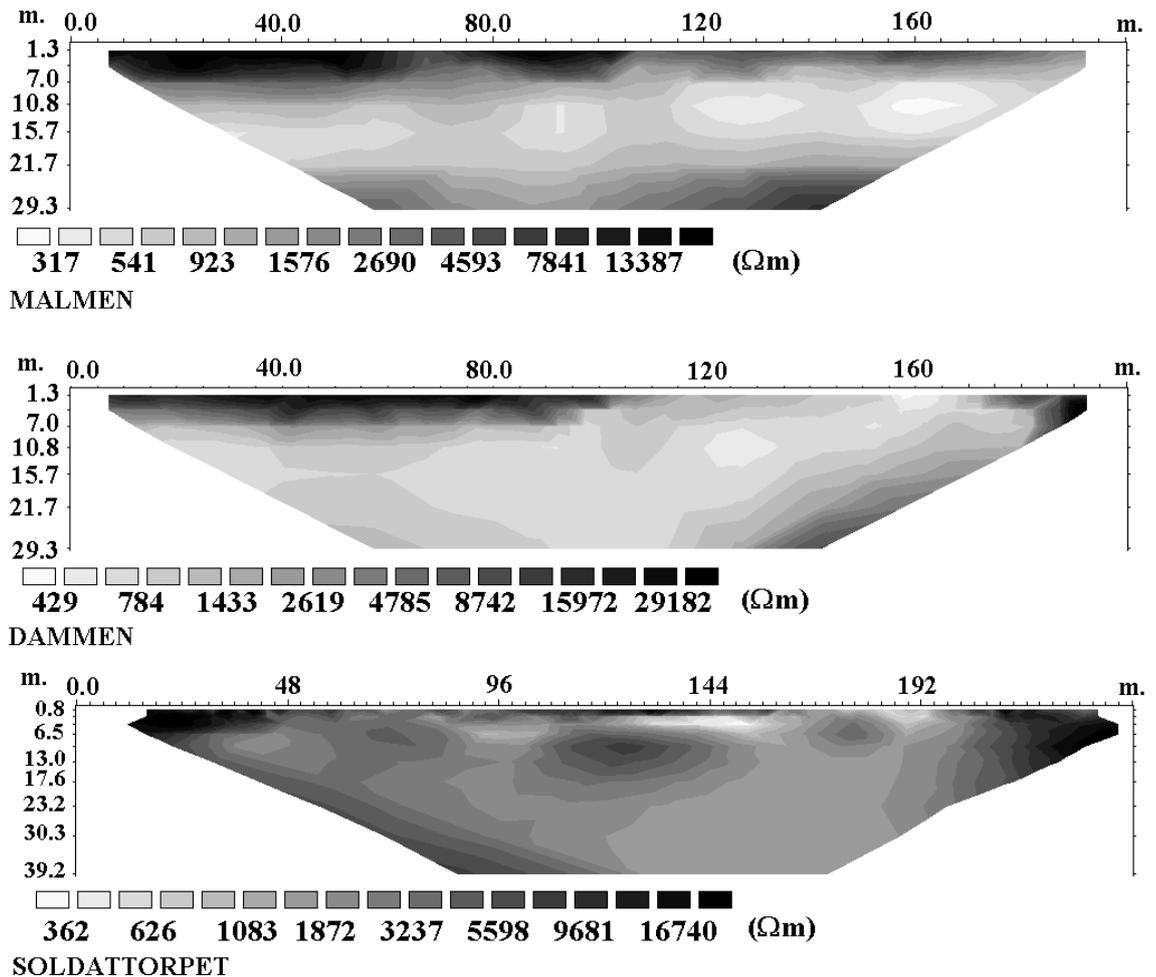
Figure 19. Resistivity inversion model sections, profiles 1 (Malmen), 2 (Dammen) and 3 (Soldattorp). Location of the profiles is given in Figure 16. All profiles are measured from north to south.
