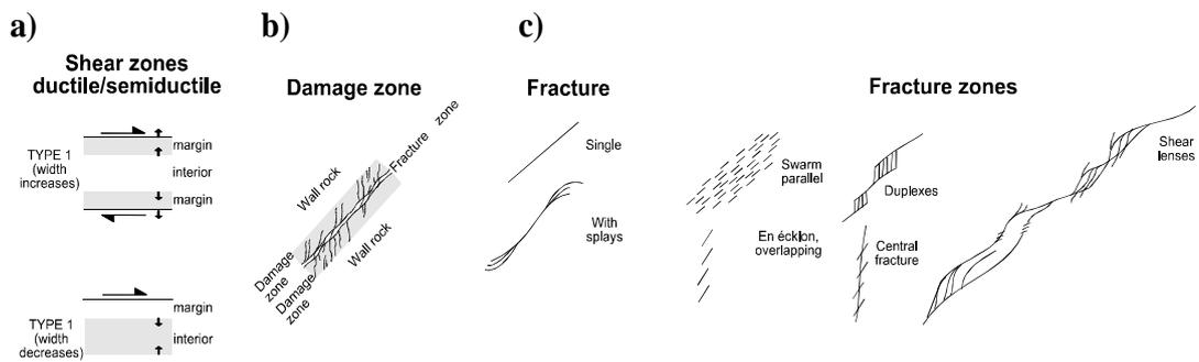
Figure 31. Geometry of deformation zones: a. deformation along shear zones (Means 1984 and 1995), b. wall rock damage zone at a shear zone or fracture zone, and c. deformation along fractures and fracture zones.
