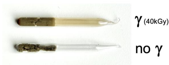
Figure 6. Photo of one glass ampule post 40 kGy irradiation and one unirradiated reference ampule.
