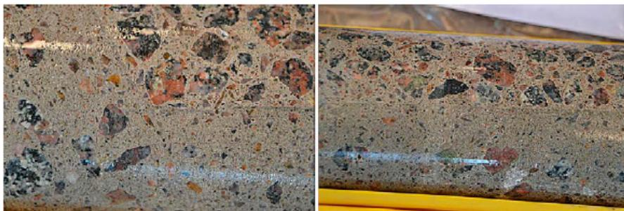
**Figure 28:** Poor aggregate distribution at wall and slab interface (SKB TR-18-12).
