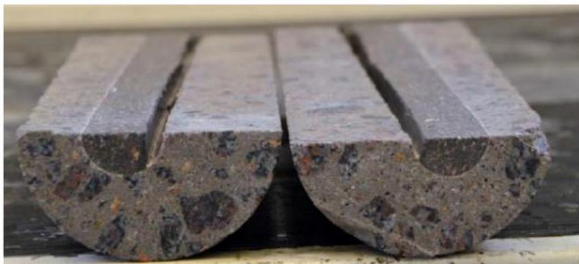
**Figure 19:** Cores through tie rod holes show incomplete grouting (SKB TR-20-09).
