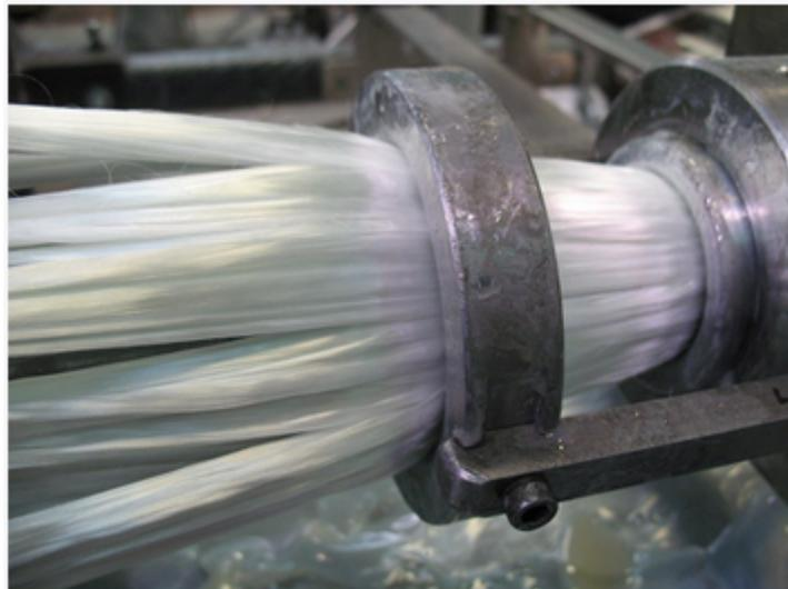
**Figure 41:** Fibre passing into pultrusion die.
