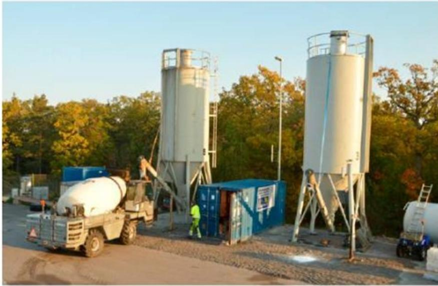
**Figure 11:** Cement and limestone powder silos (SKB TR-20-09).
