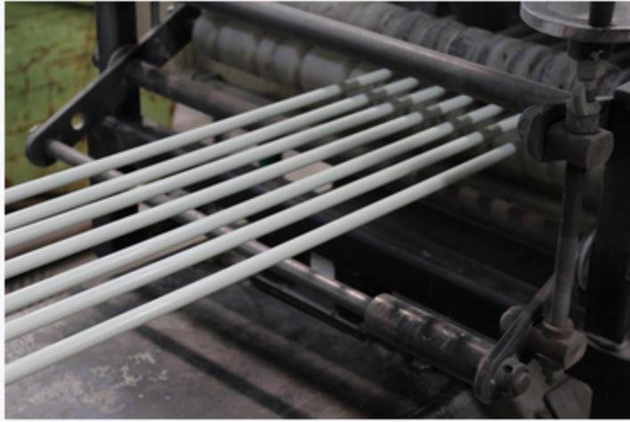
**Figure 42:** Fibre pultruded as reinforcement rods.
