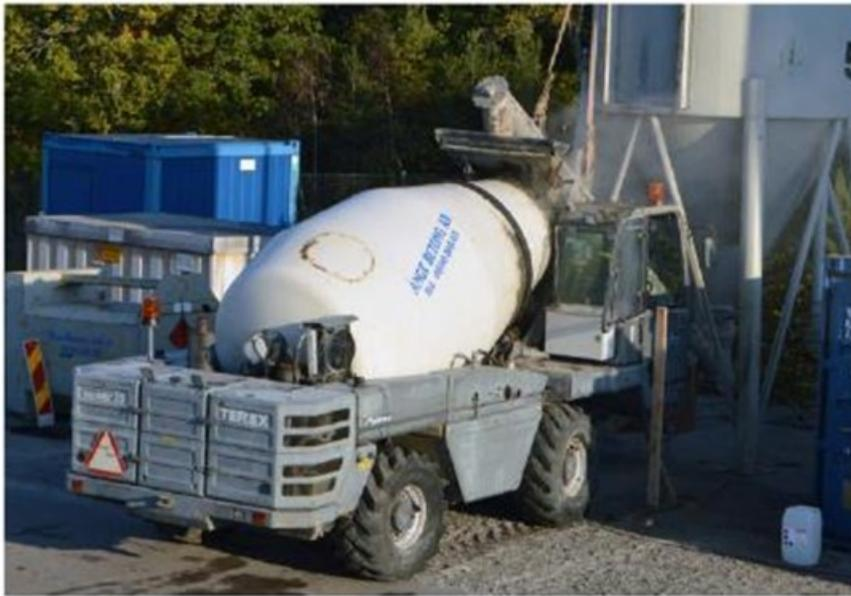
Figure 12: Feeding aggregates and powders into the truck mixer (SKB TR-20-09)
