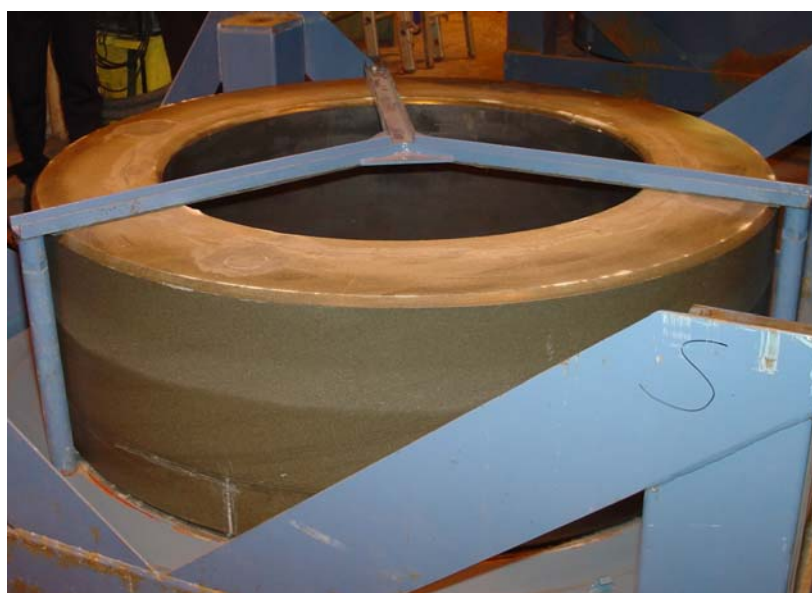
Figure 6 A ring of compressed bentonite clay that will form the buffer.
