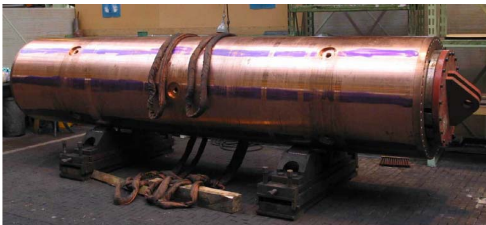
Figure 5 A modified copper canister used in the prototype repository.
