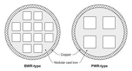
Figure 3-2. Basic differences between the BWR and PWR canister design.
