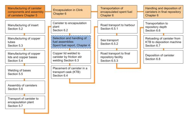
*Figure 5-1.* The main parts of the canister production line (orange) and flow chart for all stages, including references to the sections in the text where they are described. The main part presented in this chapter is highlighted.
