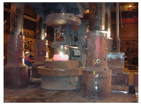
Figure 5-17. Forging of a lid blank.
