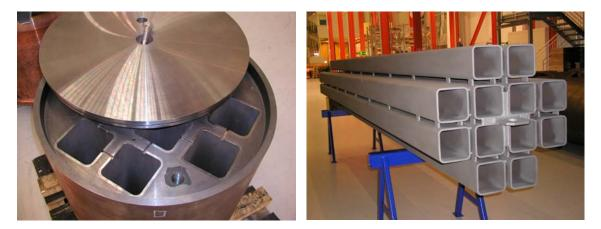
*Figure 5-4.* The photo on the left shows part of the machined insert with the notches between the fuel channels, and a steel lid with a hole for the valve for atmosphere replacement and a centre screw. The photo on the right shows a steel tube cassette.
