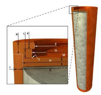
Figure 3-7. Copper shell dimensions, see Table 3-6.
