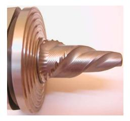
Figure 5-24. Welding tool.
