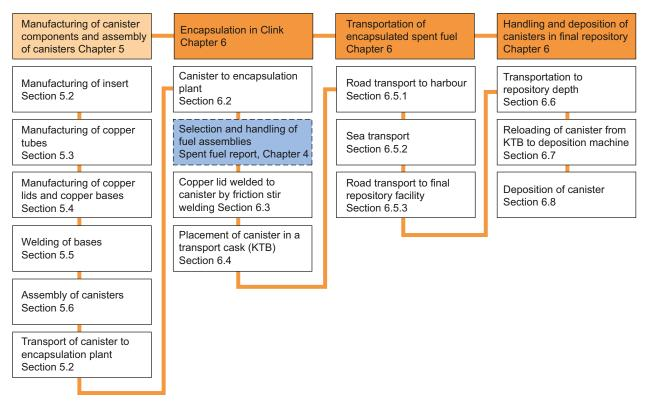
*Figure 6-1.* The main parts of the canister production line (orange) and flow chart for all stages, including references to the sections in the text where they are described. The main parts presented in this chapter are highlighted.
