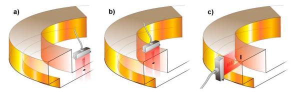
Figure 5-19. Ultrasonic testing of copper lid/base.
