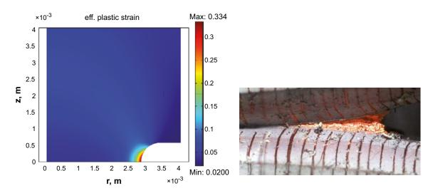
**Figure 4-7.** Left: effective plastic strain distribution after rigid-plastic deformation on notched specimen with notch acuity, a/R, equal to 5 and net section stress 215 MPa at 75°C (a is the radius of the specimen at the base of the notch and R is the notch root radius). Right: creep crack growth test with CT-specimen. An initial radius of 0.15 mm has been blunted to a radius of about 2 mm in 721 h at 150 MPa and 75°C. Vertical lines are a scale to measure potential crack growth.
