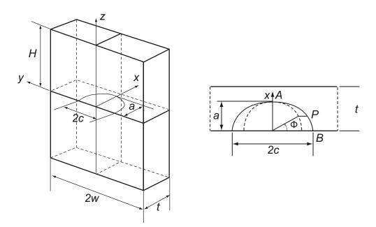
Figure 4-3. Geometry of a postulated semi-elliptical surface crack.
