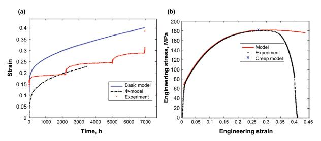
*Figure 4-1.* Comparison between models and experiment for copper; (a): copper creep models and (b): slow rate tensile testing. The jumps in the left (a) red curve are due to adjustments in the creep rig under the test as the strain was out of range.
