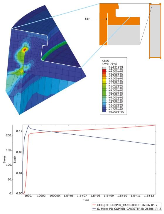
*Figure 4-8. Strain concentration to elements at the slit (top figure) and Mieses stress and equivalent creep strain for the exposed element (bottom figure).*
