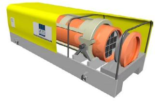
Figure 5-32. A schematic sketch of the proposed transport package for empty canisters.
