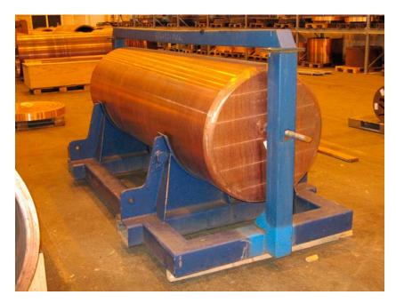
Figure 5-9. Large copper ingot weighing approximately 12 tonnes.
