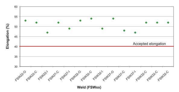
Figure 5-30. Elongation in four welds (three positions/weld) from the demonstration series.
