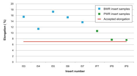
**Figure 5-6.** Elongation in BWR inserts 153-157 and PWR inserts IP7-IP9. The data shown represents the mean value of the five best samples of six according to the current manufacturing specification. For tensile test bars extracted from the top plate the accepted value in the technical specifications is 7% (shown as a red line).
