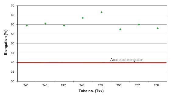
*Figure 5-13.* Elongation from samples extracted from the bottom of the copper tube (mean value of two samples). The technical specifications for test manufacturing are shown as a solid line.
