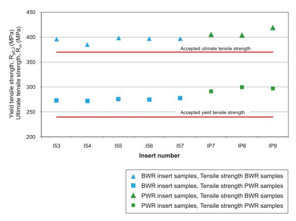
*Figure 5-7.* Yield tensile strength and ultimate strength in BWR inserts 153-157 and PWR inserts 1P7-1P9. The specified data refers to the five best samples out of six according to the current manufacturing specification. The acceptable strengths according to the technical specifications are shown as solid lines.
