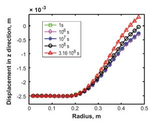
Figure 4-5. Displacement of different elements of the lid of the copper shell in axial direction.
