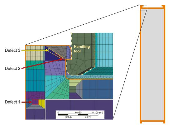
Figure 4-12. Removed volumes to model large defects.
