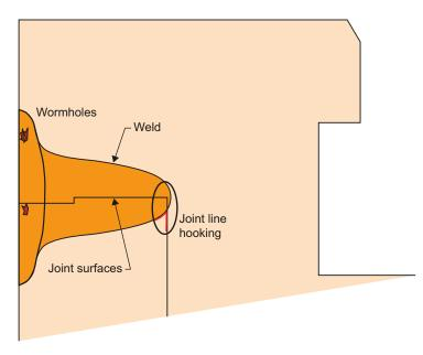
Figure 5-27. Possible defects in friction stir welds.
