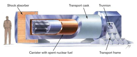
*Figure 6-3.* Schematic view of a canister in a transport cask (KTB). Trunnions in both ends of the cask are secured to the transport frame shown at the right end of the cask.
