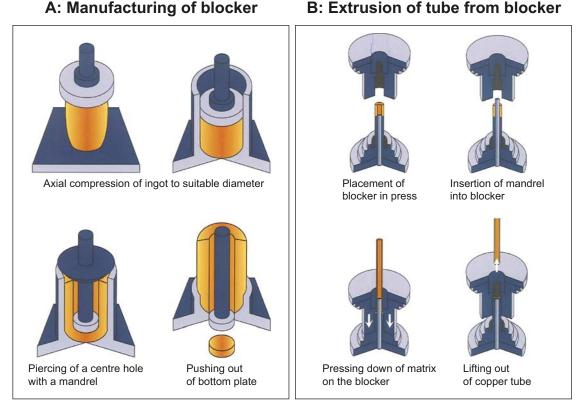
B: Extrusion of tube from blocker
