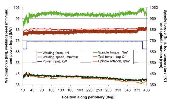
*Figure 5-29.* Weld data from lid weld. \* indicates the value of the higher y-axis. The x-axis indicates the position along the periphery in degrees.
