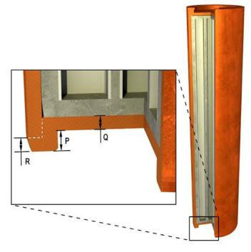
Figure 3-9. Copper base dimensions, see Table 3-6.
