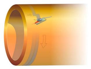
Figure 5-12. Ultrasonic testing of copper tubing by means of normal scanning.
