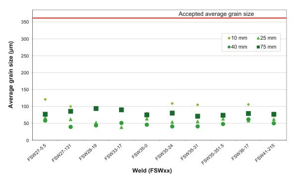
*Figure 5-31.* Average grain size in 6 welds (a total of 10 positions from the demonstration series). The different series indicate values 10, 25 and 40 mm from the surface of the canister and a reference value from the lid (75 mm).
