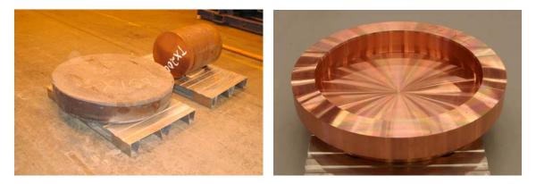
*Figure 5-18.* The photo on the left shows a small copper ingot and a forged lid blank. The photo on the right shows a machined lid.
