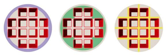
*Figure 5-5. Testing areas for BWR insert. The areas investigated with the various methods are angle scanning (lilac), normal scanning (green) and transmission testing (yellow).*
