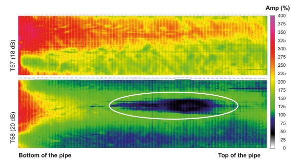
*Figure 5-15.* Results of ultrasonic testing (C-scan back-wall echo amplitude) from two extruded copper tubes. The horizontal axis represents the length of the tube, i.e.  $\sim 5$  m, whereas the vertical axis represents the circumference of the tube. The circled area shows a section with a higher level of attenuation (15 dB lower back-wall echo amplitude).
