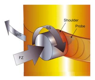
Figure 5-25. Welding parameters – spindle rotation (SS), welding force (FZ) and welding speed (WS).
