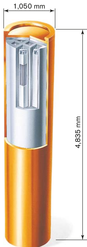
Figure 1-5. The reference design with a corrosion resistant outer copper shell and a load-bearing insert of nodular cast iron.
