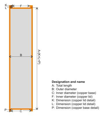
*Figure 4-6.* The dimensions of the canister determining the dimensions of the buffer blocks. The designations are the ones used in the specification of the canister reference design, see Canister production report, *Figure 3-7 to 3-9 and Table 3-6.*
