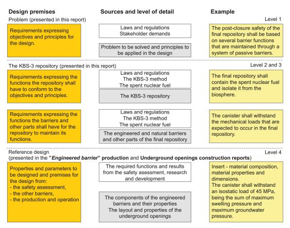
*Figure 2-1.* Different kinds of design premises, their sources and the corresponding degree of detail in the design with an example from SKB's RMS.
