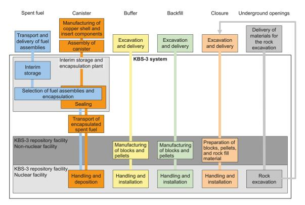
*Figure 4-5.* Overview of the main activities in the handling of the spent nucear fuel, the production of the engineered barriers and the construction of the underground openings.
