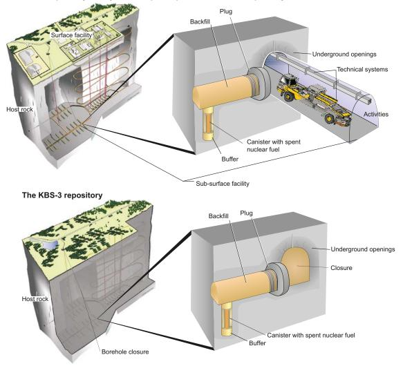
The KBS-3 repository facility with completed parts of the KBS-3 repository
