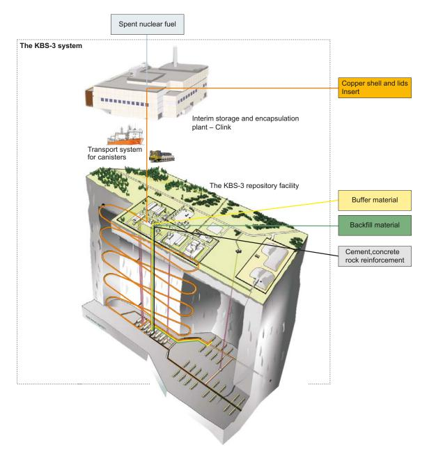
*Figure 4-1.* The KBS-3 system and its facilities and an overview of the spent fuels way through the system and the production of the KBS-3 repository.
