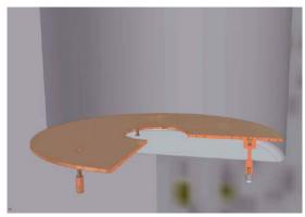
Lower copper plate resting on bolts fixed to the rock.
