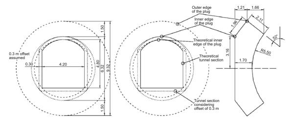
Figure 2-3. Nominal geometry for the plug.
