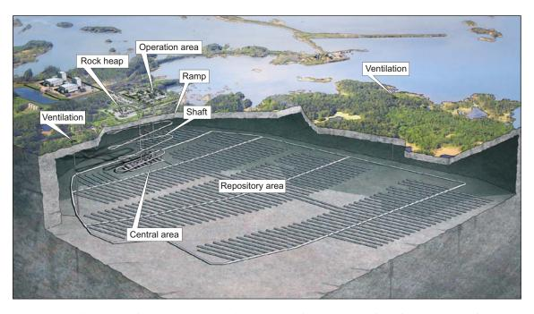
**Figure 3-1.** Illustration of the layout contained in the D2 Reference Design for a final repository facility in Forsmark.
