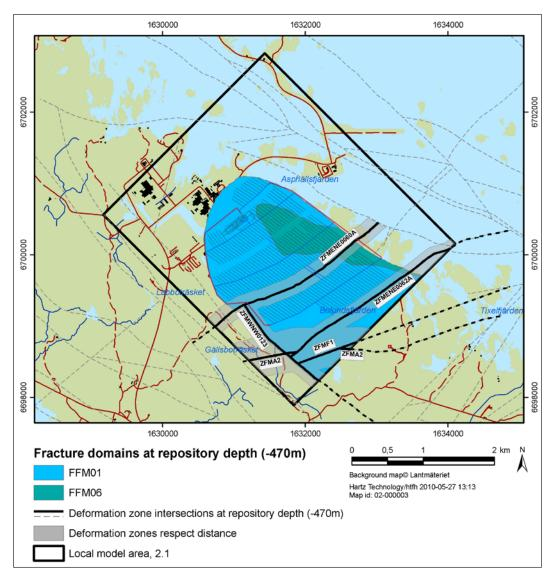
*Figure 4-1.* Deformation zones with respect distances which impact the repository layout. Section at repository depth  $(-470 \text{ m})^1$ .
