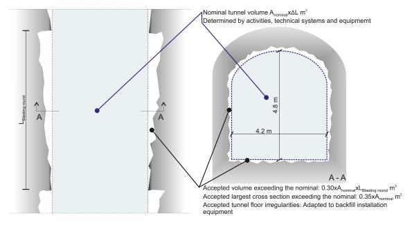
Figure 2-2. Nominal tunnel geometry and acceptable volume of rock fall out and irregularities in the tunnel walls.
