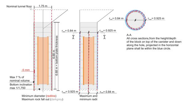
**Figure 2-1.** Nominal deposition hole geometry (black thin line) and acceptable deviations in geometry (red dotted line). The scale of the deviations in section A-A is enlarged with a factor of two. The acceptable deviations concern the part of the deposition hole where the buffer is going to be installed. The top of the deposition hole is designed with respect to operational requirements.
