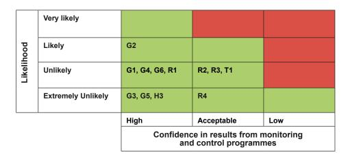
**Figure 6-2.** Risk matrix showing likelihood of occurrence for the identified hazards and the confidence in detecting that the initial state of underground openings does not conform to the design premises listed in Section 6.4.4.
