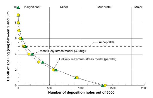
Figure 4-3. Loss of deposition holes for the "Most likely" stress model with the deposition tunnels at 30 degrees to the maxim horizontal stress and the "Unlikely maximum" stress model with the deposition tunnel parallel to the maximum horizontal stress /SKB 2009b/.
