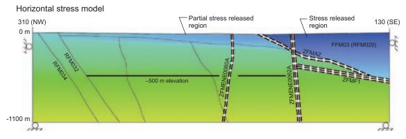
**Figure 4-19.** Comparison of fracture domain, hydrogeological DFN and maximum horizontal stress models along a NW-SE profile in the north-western part of the candidate volume (Figure 11-21 in the **Site description Forsmark**).
