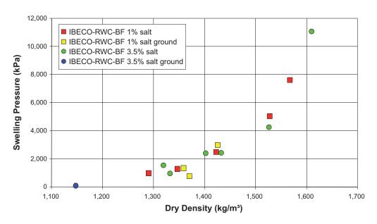
Figure 5-19. The swelling pressure of Ibeco RWC-BF as function of the dry density; "ground" refers to a material that was re-milled before compaction /Johannesson et al. 2010/.
