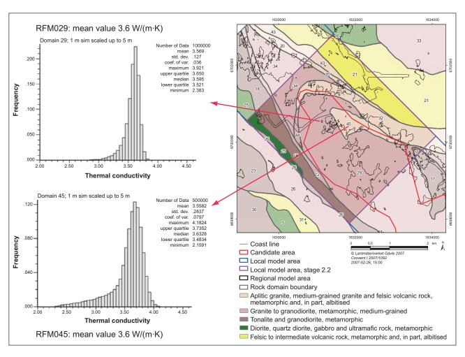
**Figure 4-9.** Modelled thermal conductivity at the 5 m scale. The lower tail of the distribution is mainly due to the subordinate rock type amphibolite (Figure 11-10 in the **Site description Forsmark**).
