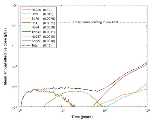
**Figure S-11.** Probabilistically calculated consequences of shear failure, for the period between 1,000 years and one million years. The legends are sorted according to descending peak mean annual effective dose over one million years (given in brackets in  $\mu$ Sv).
