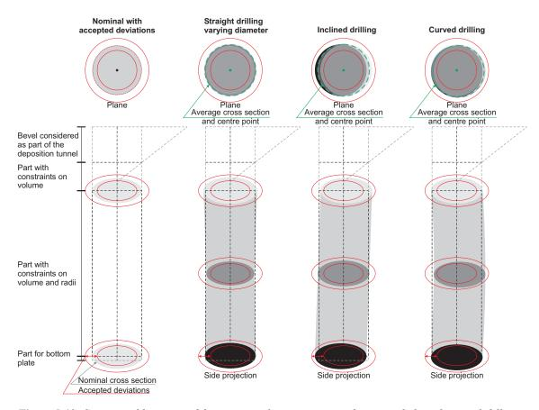
**Figure 5-13.** Some possible causes of deviations in the geometry in a deposition hole without rock fall out. All kinds of deviations can occur in the same deposition hole. The deviations are exaggerated in scale. (The bevel is discussed in the backfilling section).
