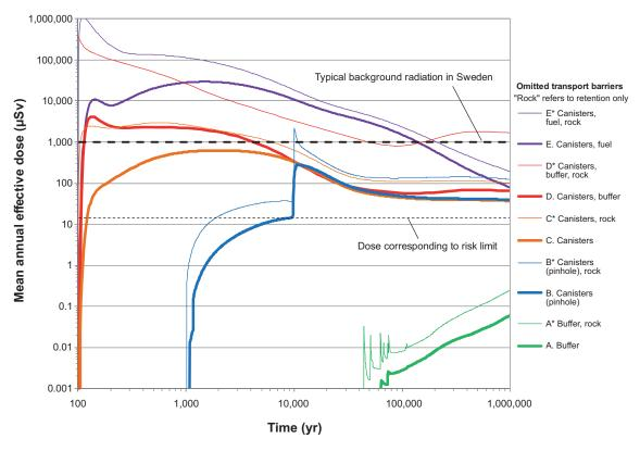
**Figure S-12.** Results of stylised cases to illustrate loss of barrier functions. Note that an omission of the "rock" barrier in these cases refers to omission of retention of radionuclides in the rock fractures only, whereas the favourable, low flow rate at repository depth and the favourable geochemical conditions are still taken into account.
