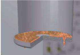
Concrete slab poured through the hole in the centre of the lower copper plate.
