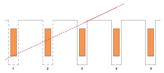
**Figure 5-4.** In SR-Site, the EFPC criterion is changed such that deposition positions being intersected by a fracture that intersects the full tunnel perimeter and that also is projected to intersect the canister location in the deposition hole, are rejected (i.e. positions 1 and 2). For potentially water bearing fractures the previous criterion still applies (i.e. position 3 is also rejected).
