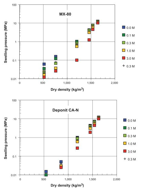
*Figure 5-14.* Swelling pressures of MX-80 exposed to NaCl solutions (upper) and Ibeco RWC (Deponit CA-N) exposed to CaCl<sub>2</sub> solutions (lower). Concentration expressed as M.
