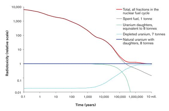
**Figure S-2.** Radiotoxicity on ingestion of uranium and daughters in ore (blue line), and of the sum of all fractions that arise when the same quantity of uranium is used in the nuclear fuel cycle (red line). The time refers to the time after reactor operation. The different fractions comprise the spent fuel (38 MWd thermal energy/kg U of type SVEA 64 BWR), the depleted uranium and the uranium daughters that are separated in the uranium mill.
