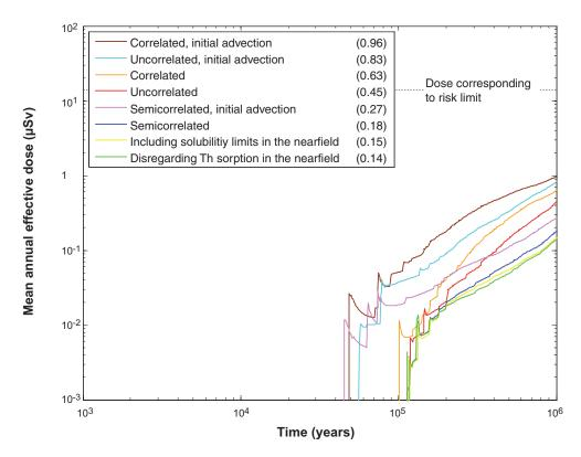
**Figure S-10.** Summary of far-field mean annual effective dose for all probabilistic calculations performed for the corrosion scenario. The peak doses are given in parentheses in  $\mu$ Sv. In the legend, 'Correlated', 'Uncorrelated' and 'Semicorrelated' refer to three variants of the hydrogeological model used in SR-Site. The three 'initial advection' cases put upper bounds on the possible consequences of buffer erosion.
