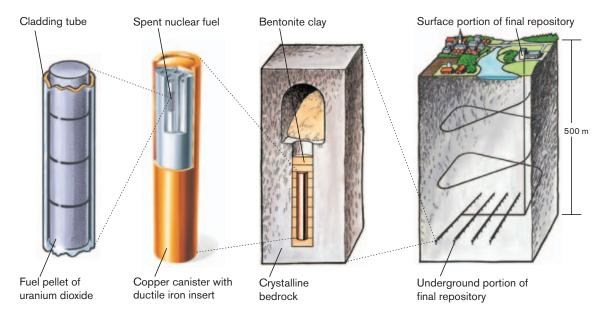
Figure 5-2. The KBS-3 concept for storage of spent nuclear fuel.
