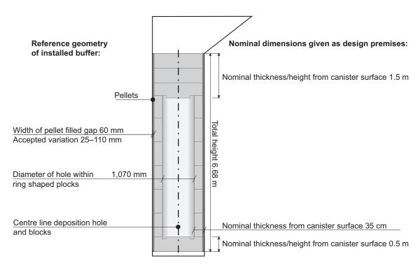
Figure 5-11. Reference geometry of the installed buffer, see the Buffer production report, Figure 3-3.
