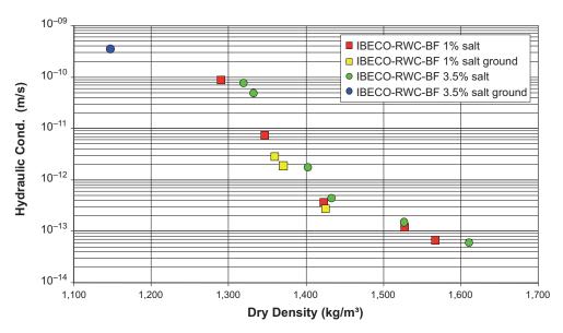
Figure 5-18. The hydraulic conductivity of Ibeco RWC-BF as function of the dry density; "ground" refers to a material that was re-milled before compaction /Johannesson et al. 2010/.
