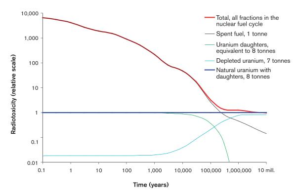
**Figure 2-1.** Radiotoxicity on ingestion of uranium and daughters in ore (blue line), and of the sum of all fractions that arise when the same quantity of uranium is used in the nuclear fuel cycle (red line). The time refers to the time after reactor operation. The different fractions comprise the spent fuel (38 MWd thermal energy/kg U of type SVEA 64 BWR), the depleted uranium and the uranium daughters that are separated in the uranium mill. From /Hedin 1997/.
