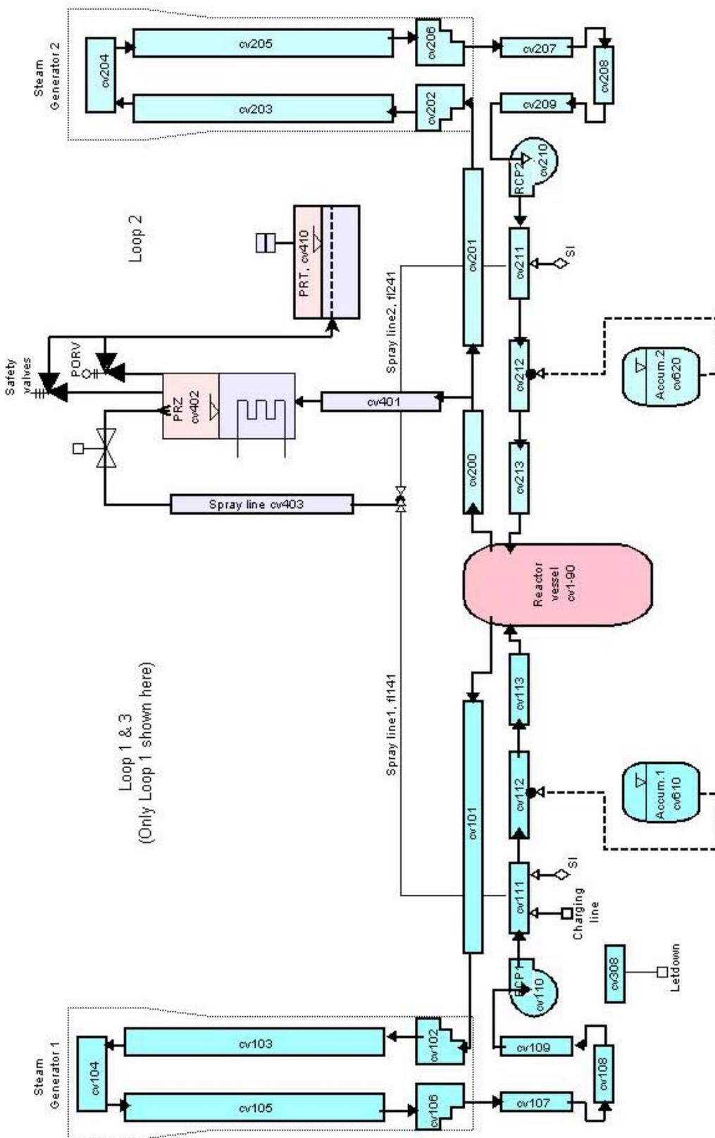
Figure 7. Nodalization scheme for the primary system cooling loops
