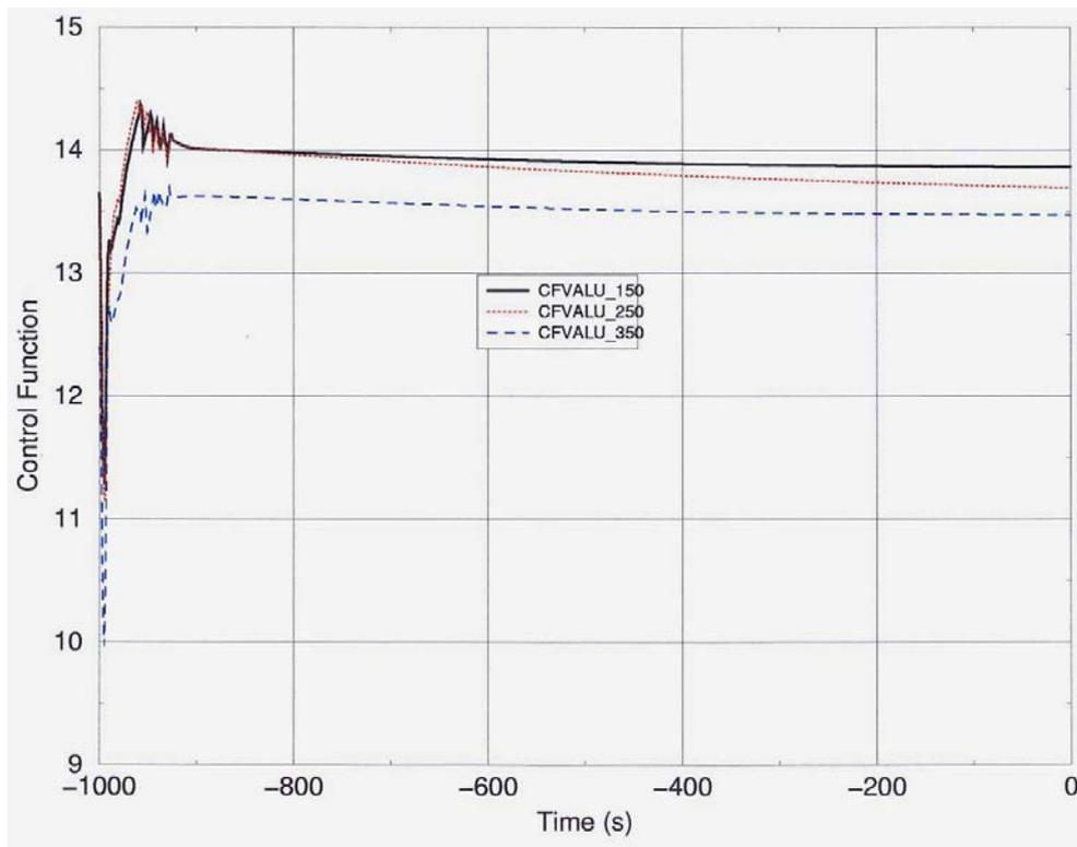
Figure 16. Water Level in Downcomer above Tube Plate, Steam Generator 1-3
