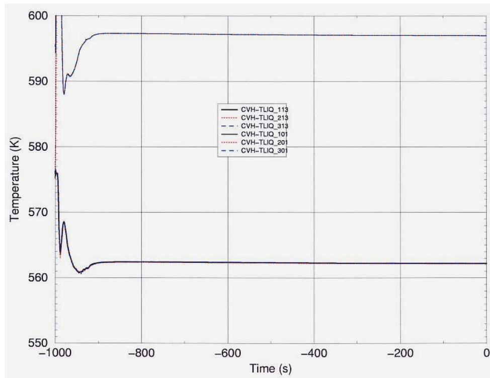
Figure 14. Primary Loop Temperatures in Cold and Hot Legs
