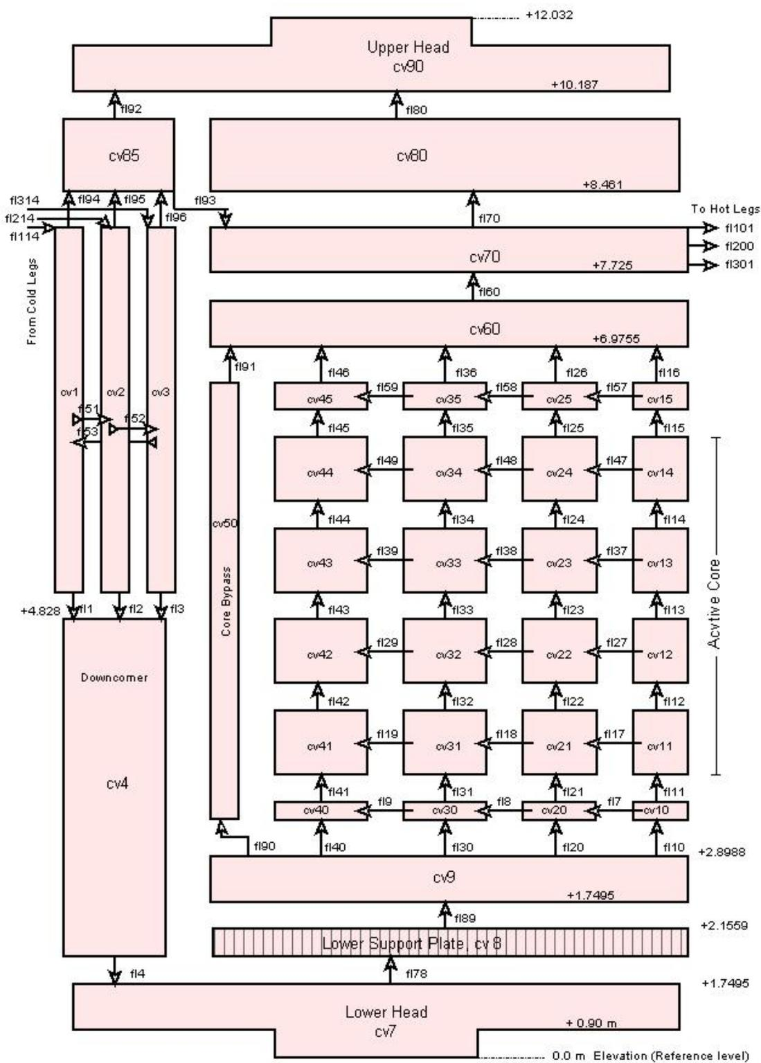
Figure 5. Nodalization scheme for the reactor vessel
