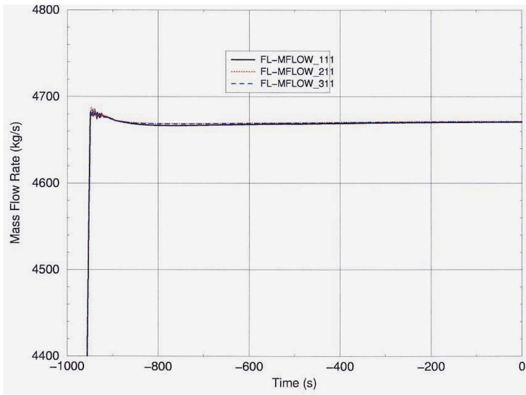
Figure 12. Recirculation Mass Flow Rate in Primary Loop
