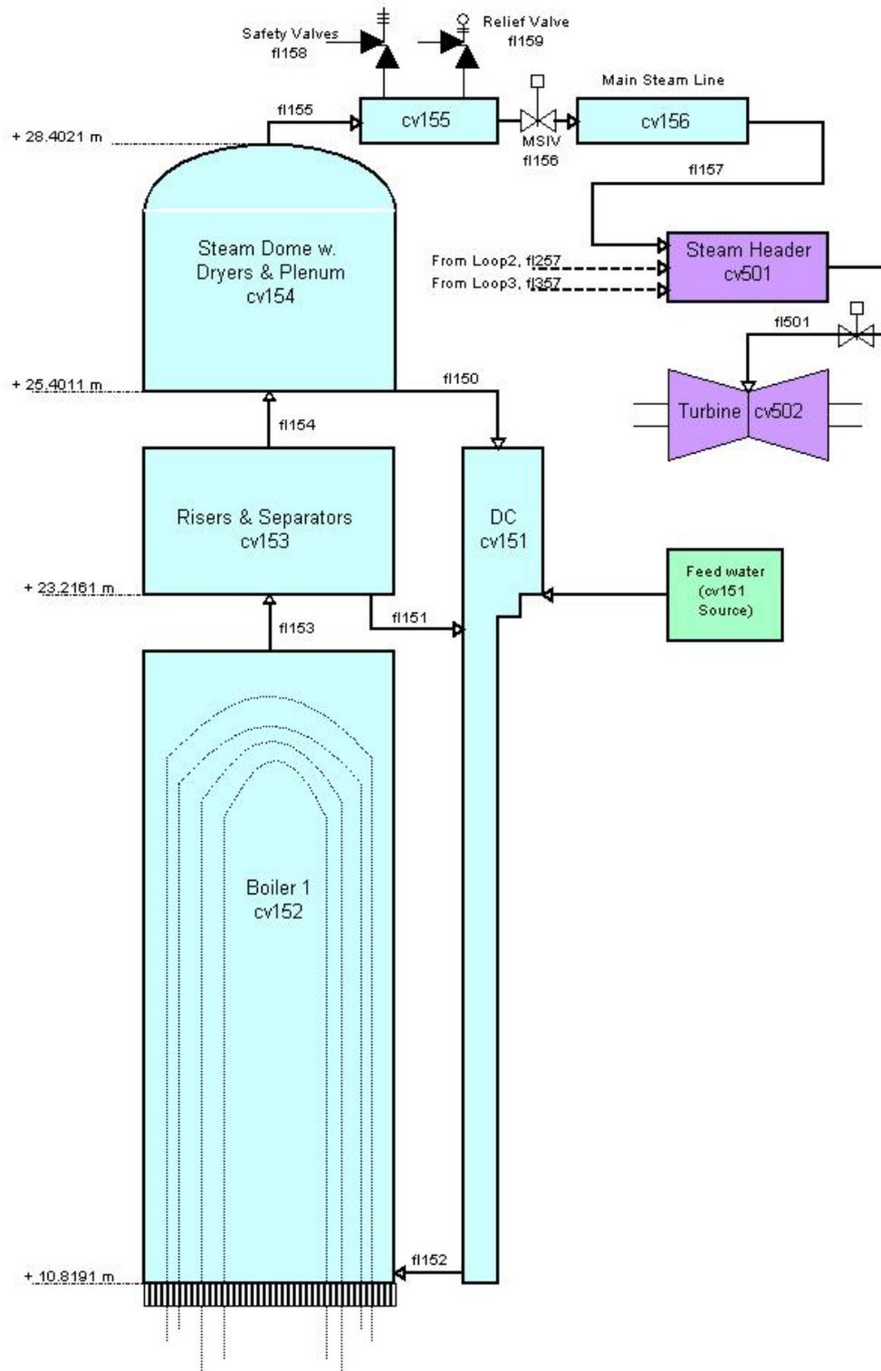
Figure 8. Nodalization of the secondary system
