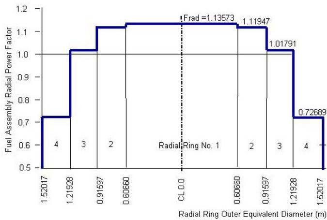
Figure 4. Radial power distribution per assembly in the radial rings, normalized.
