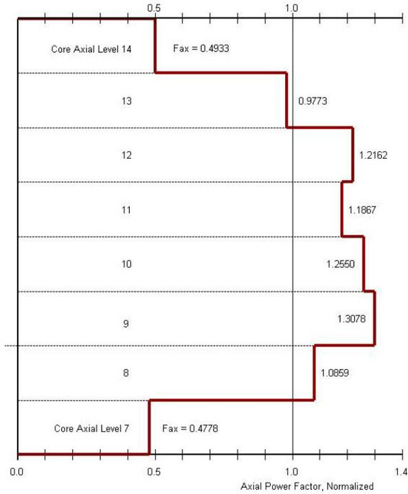
Figure 3. Axial power distribution used in the MELGEN COR input.
