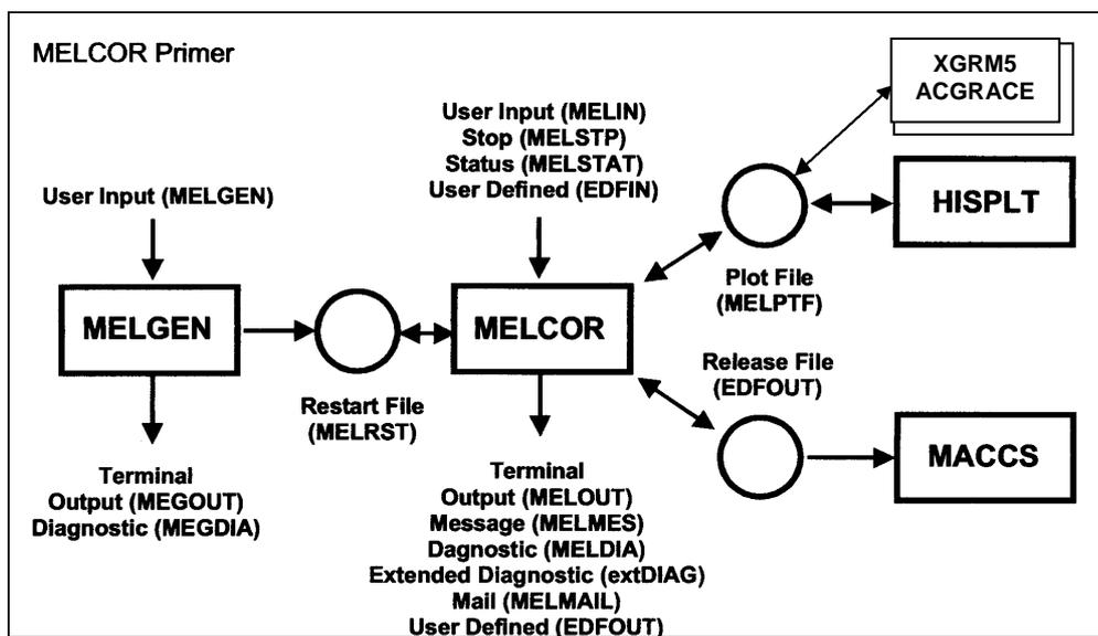
Figure 1. Relationship between the various codes and files in MELCOR
