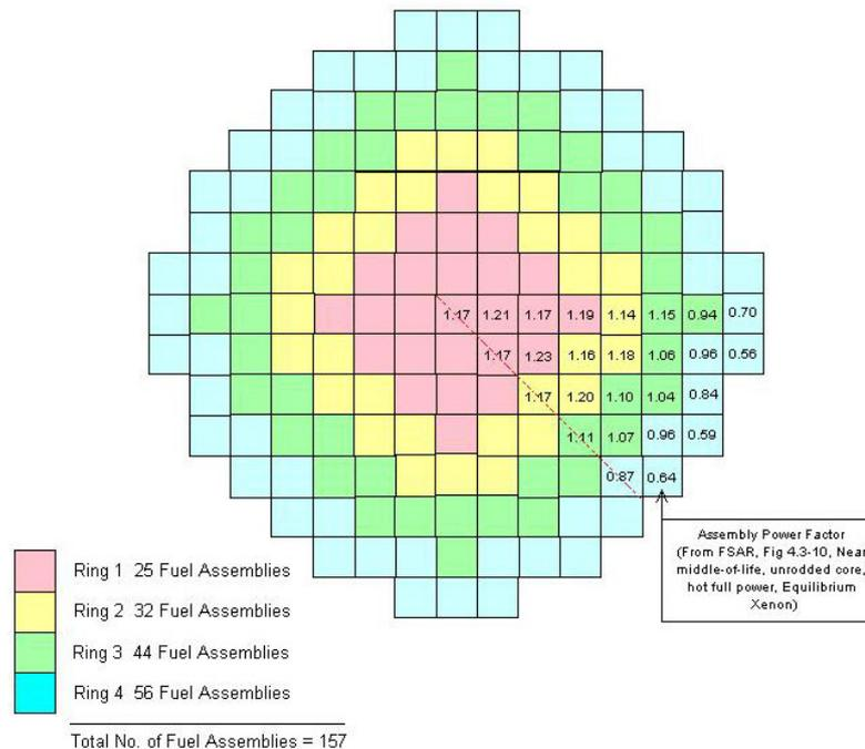
Figure 2. Cross section of core showing distribution of fuel assemblies into the radial rings and assembly power factors for 1/8 symmetry.
