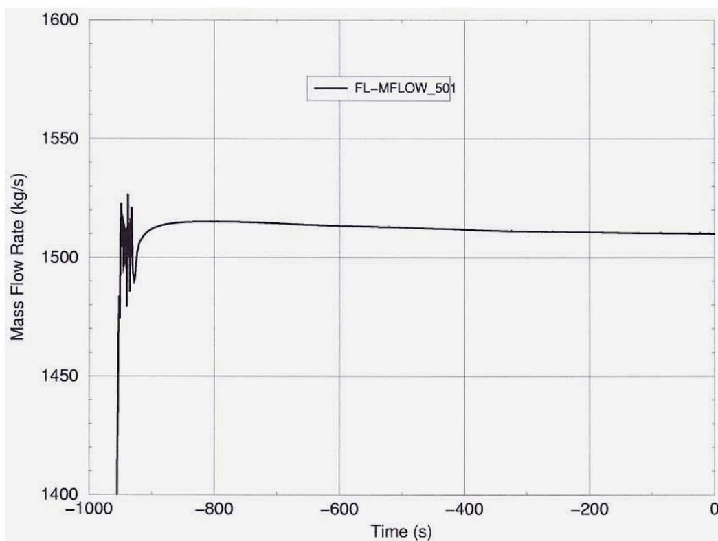
Figure 13. Steam Mass Flow Rate to Turbine
