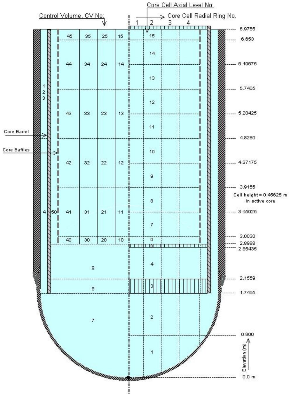
Figure 6. Nodalization of the core
