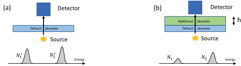
Figure 3. Schematic view of an experimental setup consisting of a point source, an absorbing layer, and a detector. (a) Calibration configuration. (b) Measurement configuration. An additional layer with the thickness of h is added to the calibration configuration.
