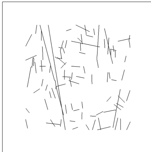
Figure A2.13. DFN realisation FFM01geoDFNr0fixed04_N35W2d.prn. 96 fractures larger than 3 m were extracted from the large data set. The vertical cross section faces NE in direction of Sh.
