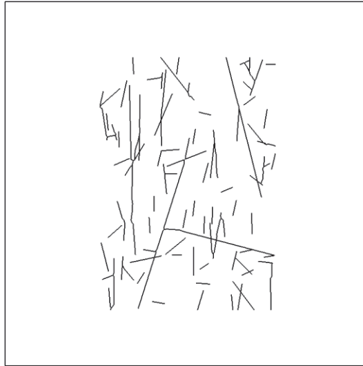
Figure A2.20. DFN realisation FFM01geoDFNr0fixed06_N55E2d.prn. 99 fractures larger than 3 m were extracted from the large data set. The vertical cross section faces SE in direction of SH.
