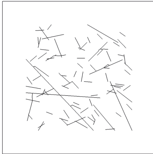
Figure A2.12. DFN realisation FFM01geoDFNr0fixed04_HZ2d.prn. 88 fractures larger than 3 m were extracted from the large data set. The horizontal cross section faces in direction of Sv.
