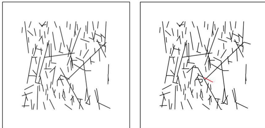
Figure 4.17. Vertical N35W section. (Left) Initial fracture geometry of FFM01geoDFNr0fixed02_N35W2d (SH-SV plane, SH is horizontal). (Right) Fracture propagation in the final simulation step 10. The initial total fracture length increases by 3.4%.
