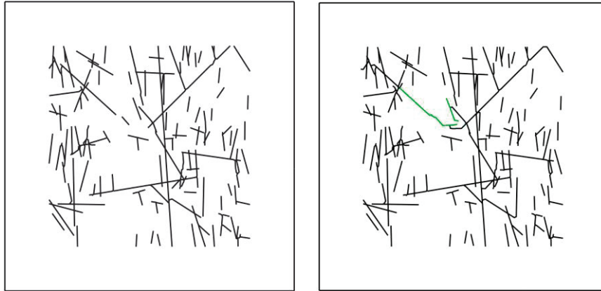
Figure 4.5. Vertical N35W section. (Left) Initial fracture geometry of FFM01geoDFNr0fixed06_N35W2d (SH-SV plane, SH is horizontal). (Right) Fracture propagation in the final simulation step 8. The initial total fracture length increases by 2.1%.
