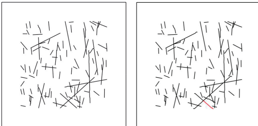
Figure 4.20. Vertical N35W section. (Left) Initial fracture geometry of FFM01geoDFNr0fixed07_N35W2d (SH-SV plane, SH is horizontal). (Right) Fracture propagation in the final simulation step 6. The initial total fracture length increases by 1.7%.
