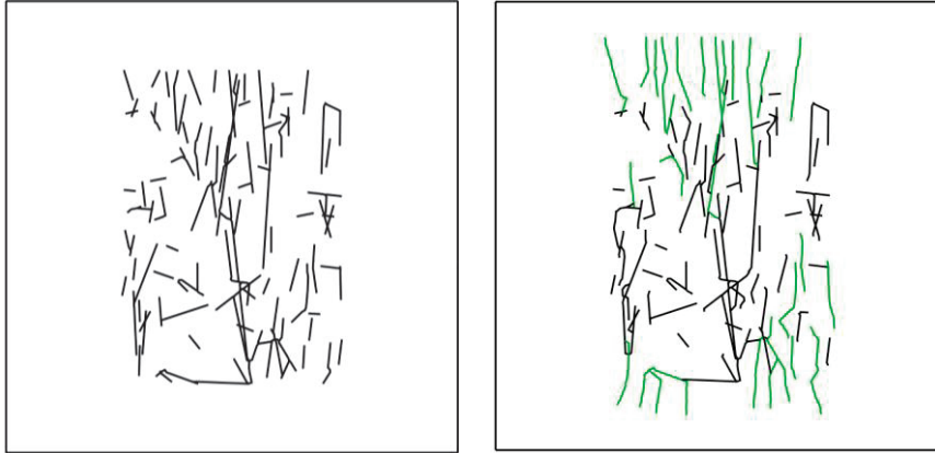
Figure 6.24. Vertical N55E section. (Left) Initial fracture geometry of FFM01geoDFNr0fixed08_N55E2d (Sh-SV plane, Sh is horizontal). (Right) Fracture propagation in the final simulation step 10. The initial total fracture length increases by 29.2%.
