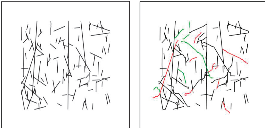
Figure 3.8. Vertical N35W section. (Left) Initial fracture geometry of FFM01geoDFNr0fixed10_N35W2d (SH-SV plane, SH is horizontal). (Right) Fracture propagation in the final simulation step 10. The initial total fracture length increases by 19.3%.
