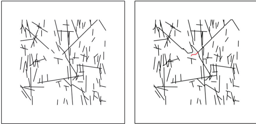
Figure 6.15. Vertical N35W section. (Left) Initial fracture geometry of FFM01geoDFNr0fixed06_N35W2d (SH-SV plane, SH is horizontal). (Right) Fracture propagation in the final simulation step 10. The initial total fracture length increases by 2.1%.
