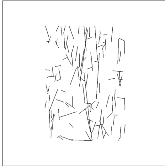
Figure A2.26. DFN realisation FFM01geoDFNr0fixed08_N55E2d.prn. 117 fractures larger than 3 m were extracted from the large data set. The vertical cross section faces SE in direction of SH.
