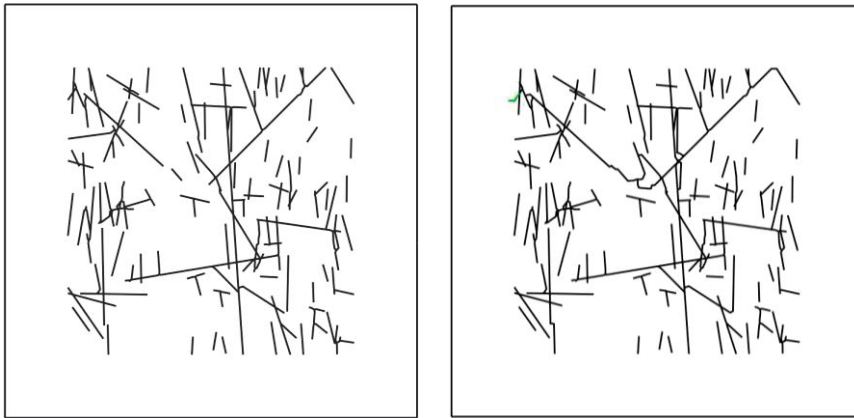
Figure 4.19. Vertical N35W section. (Left) Initial fracture geometry of FFM01geoDFNr0fixed06_N35W2d (SH-SV plane, SH is horizontal). (Right) Fracture propagation in the final simulation step 10. The initial total fracture length increases by 2.3%.
