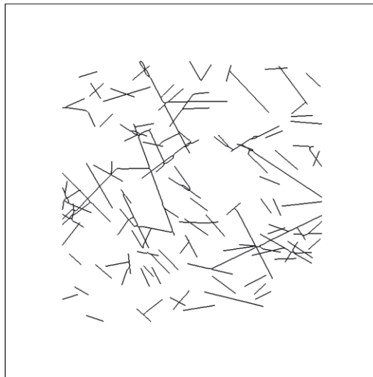
Figure A2.27. DFN realisation FFM01geoDFNr0fixed09_HZ2d.prn. 135 fractures larger than 3 m were extracted from the large data set. The horizontal cross section faces in direction of Sv.
