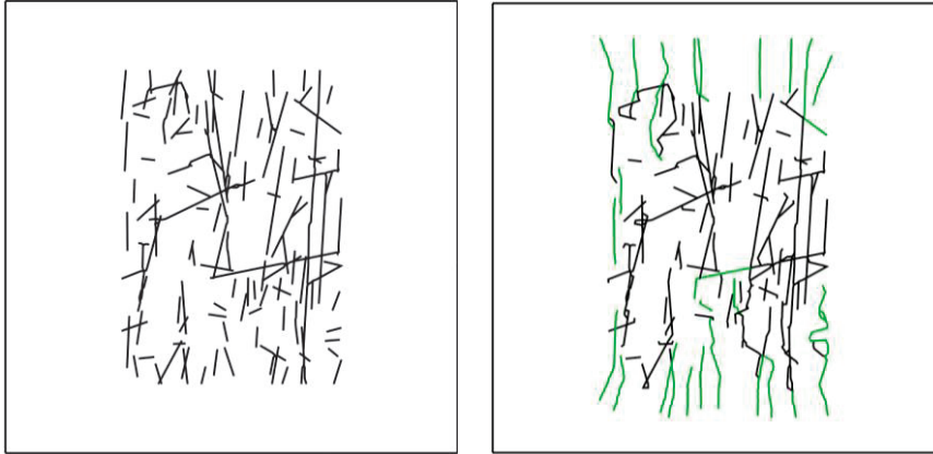
Figure 6.18. Vertical N55E section. (Left) Initial fracture geometry of FFM01geoDFNr0fixed01_N55E2d (Sh-SV plane, Sh is horizontal). (Right) Fracture propagation in the final simulation step 10. The initial total fracture length increases by 27.8%.
