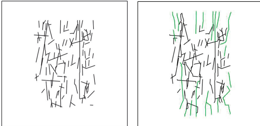
Figure 6.25. Vertical N55E section. (Left) Initial fracture geometry of FFM01geoDFNr0fixed09_N55E2d (Sh-SV plane, Sh is horizontal). (Right) Fracture propagation in the final simulation step 10. The initial total fracture length increases by 29.4%.
