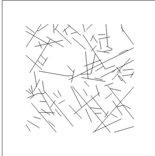
Figure A2.6. DFN realisation FFM01geoDFNr0fixed02_HZ2d.prn. 107 fractures larger than 3 m were extracted from the large data set. The horizontal cross section faces in direction of Sv.
