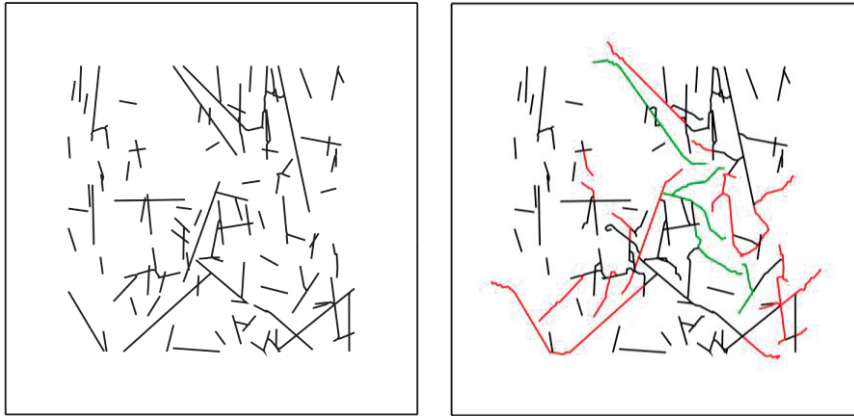
Figure 3.6. Vertical N35W section. (Left) Initial fracture geometry of FFM01geoDFNr0fixed08_N35W2d (SH-SV plane, SH is horizontal). (Right) Fracture propagation in the final simulation step 10. The initial total fracture length is increased by 25.4%.
