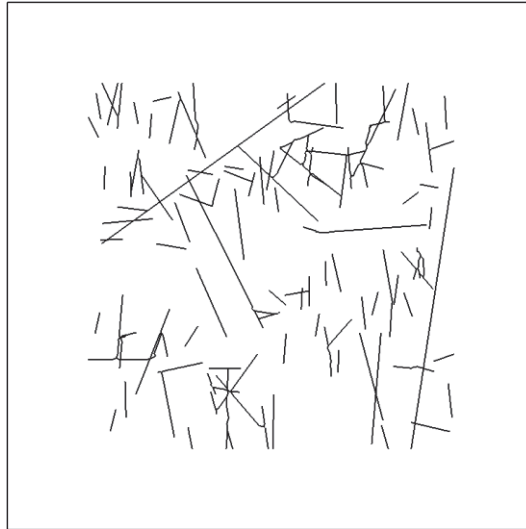
Figure A2.10. DFN realisation FFM01geoDFNr0fixed03_N35W2d.prn. 125 fractures larger than 3 m were extracted from the large data set. The vertical cross section faces NE in direction of Sh.
