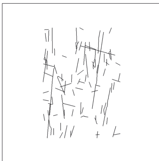
Figure A2.14. DFN realisation FFM01geoDFNr0fixed04_N55E2d.prn. 103 fractures larger than 3 m were extracted from the large data set. The vertical cross section faces SE in direction of SH.
