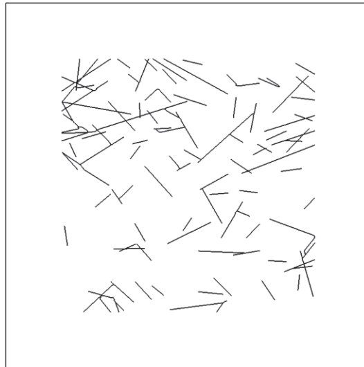
Figure A2.3. DFN realisation FFM01geoDFNr0fixed01_HZ2d.prn. 107 fractures larger than 3 m were extracted from the large data set. The horizontal cross section faces in direction of Sv.
