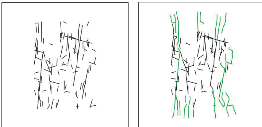
Figure 6.20. Vertical N55E section. (Left) Initial fracture geometry of FFM01geoDFNr0fixed04_N55E2d (Sh-SV plane, Sh is horizontal). (Right) Fracture propagation in the final simulation step 10. The initial total fracture length increases by 35.5%.
