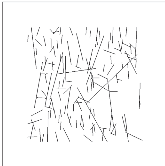
Figure A2.7. DFN realisation FFM01geoDFNr0fixed02_N35W2d.prn. 135 fractures larger than 3 m were extracted from the large data set. The vertical cross section faces NE in direction of Sh.
