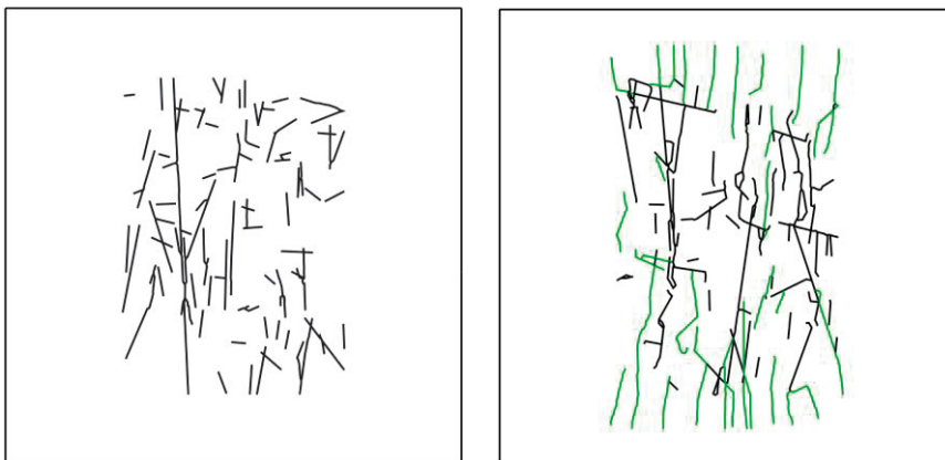
Figure 6.26. Vertical N55E section. (Left) Initial fracture geometry of FFM01geoDFNr0fixed10_N55E2d (Sh-SV plane, Sh is horizontal). (Right) Fracture propagation in the final simulation step 10. The initial total fracture length increases by 29.8%.
