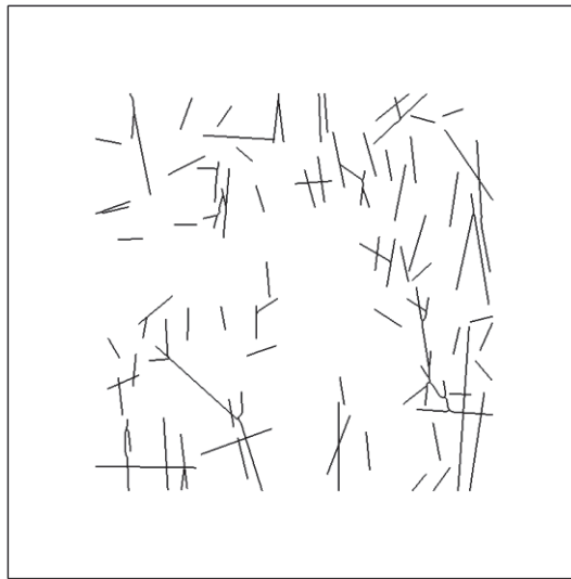
Figure A2.4. DFN realisation FFM01geoDFNr0fixed01_N35W2d.prn. 102 fractures larger than 3 m were extracted from the large data set. The vertical cross section faces NE in direction of Sh.
