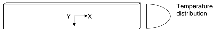
Figure 5. A verification case with a thin rectangular plate with temperature distribution (from Timoshenko and Goodier, 1970). Boundaries are free to move in this verification study. Another case with a thick plate was also tested with good results.
