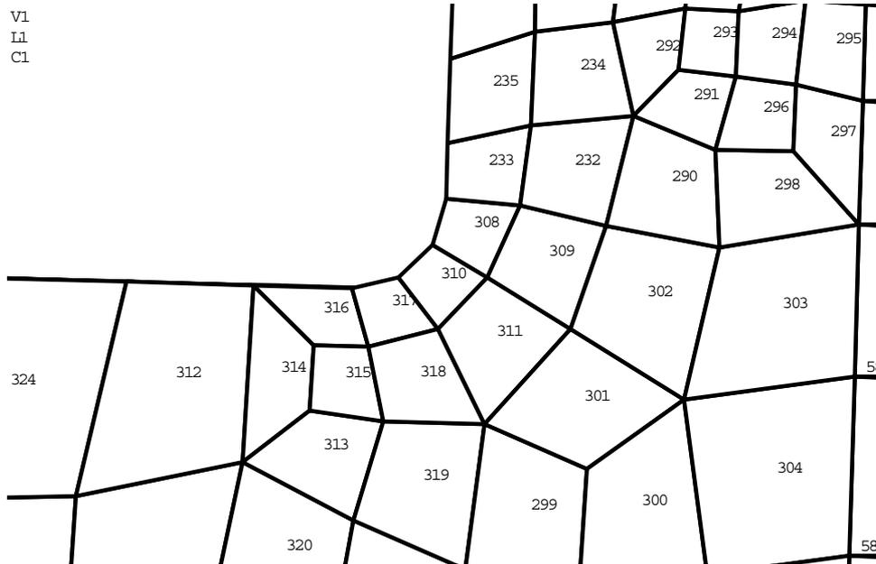
Figure 101 Elements in the lid fillet region for axisymmetric analyses.
