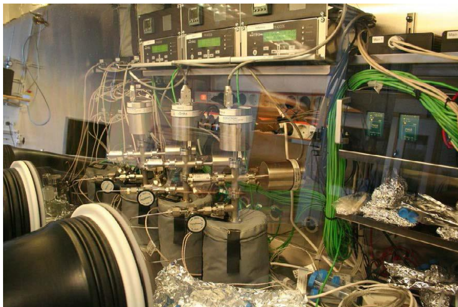
Figure 3: The three experiments in the glove box, showing the heating jacket around each reaction chamber and the vacuum chamber with pressure gauge above the reaction chamber (Boman et al., 2014).
