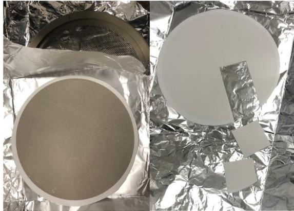
**Figure 7** Aerosol-laden filter collected with a HiVol DHA-80 sampler (Digitel) at Hyltemossa research station with a flow rate of  $\sim 36 \text{ m}^3 \text{ h}^{-1}$  (see [42] for further details). The filter diameter is 15 cm of which 14 cm is exposed (filter 3 in
