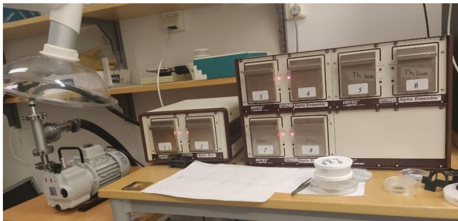
**Figure 8** The alpha detector setup used for measurement of the membrane filters.
