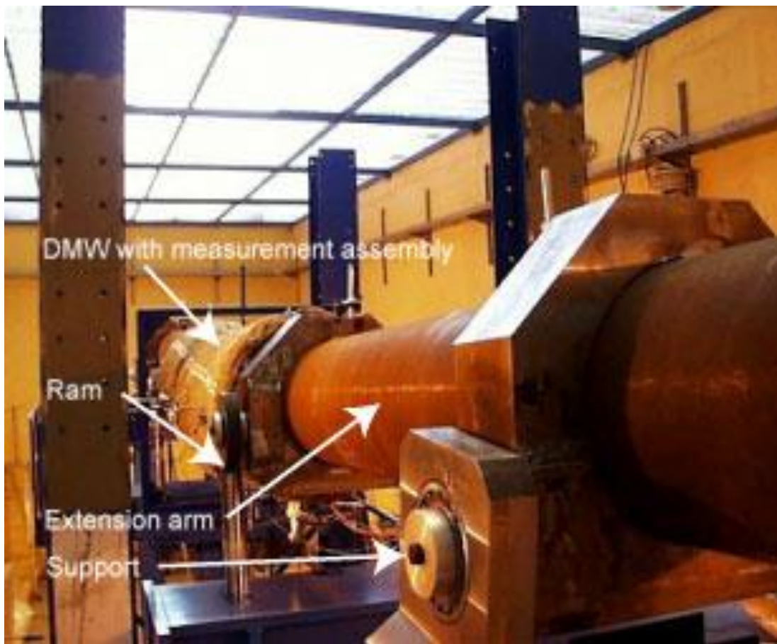
Fig. 3.1: Four-point bending assembly used by EdF at Les Renardières in France.
