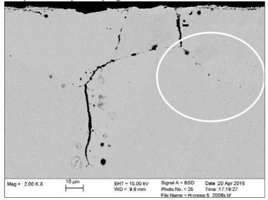
Figure 3-8. Specimen H-creep-05 tested at RT for 1005.7 hours hydrogen charging time and creep stress of 170 MPa. Larger cracks were discovered. The specimen was tested in soft annealed condition without any pre-strain.
