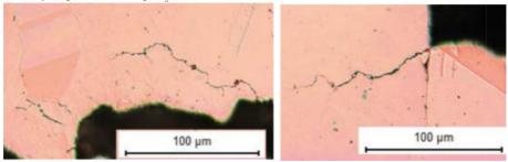
**Figure 3.15**. Details from Figure 4-7 in /Gordon A. et al. 2017/. Middle part of pre-crack of WOL sample M4 4:1 (MiniCan 4), showing smaller cracks emanating perpendicular to the direction of the main crack.
