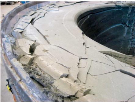
Figure 2.5. From SKB-report TR-17-15, Fig 2.9. SKB has shown in several reports that it is impossible to add water to bentonite blocks without severe cracking under normal pressure.
