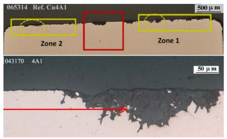
Figure 4.6. Metallographic cross-sections showing the exposed copper sample with pitting corrosion, up to  $100\mu m$  in depth. From Appendix B in the FEBEX-report /Wersin P. and Kober F 2017/.
