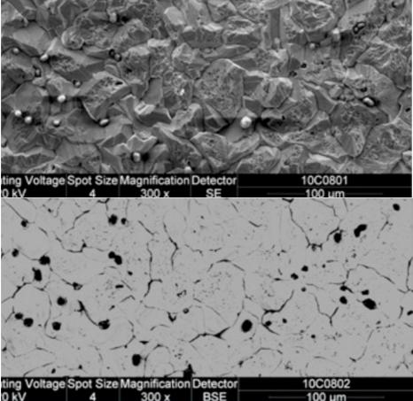
**Figure 3.14**. Detail from Figure 4 in /Arilahti E. et al 2011/. The SEM-image at the top shows a post exposure fractured area ahead of the true crack tip for which EDS analysis showed average of 22.5 at-% sulphur. The backscatter electron image of the same area (bottom picture) shows darker sulphur-rich precipitates mostly at the grain boundaries.
