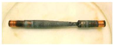
Figure 3.3. Example of SSRT exposed sample, 9 % strain at the thinnest part of the tapered sample (not exposed to final fracture).
