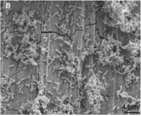
**Figure 3.18.** Microbial corrosion on the surface of unalloyed copper creates micro cracks due to sulphur enrichment. SRB colonies convert sulphate to sulphide which results in SCC/ Carpén L. et al. 2016/.
