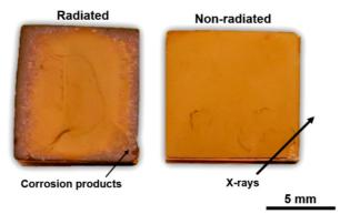
**Figure 5.2.** Photograph of some of the copper samples to be investigated. The radiated specimen in this case was exposed to oxygen-free water for 64 hours with a simultaneous exposure to 28.6 kGy of gamma radiation. The non-radiated specimen was exposed to oxygen-free water for 64 hours only. The bar shows the scan direction of x-rays through the specimen.
