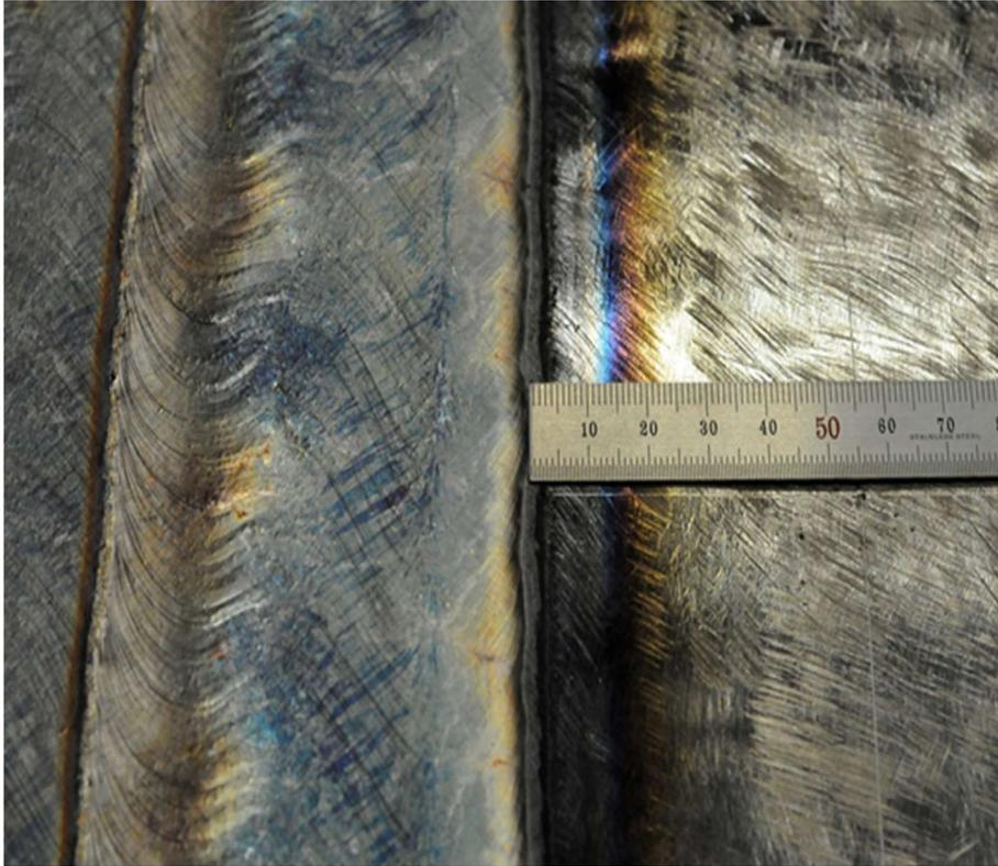
Figure 3 The submerged arc strip cladding process resulted in deposited beads of approximately 70 mm width and 5 mm build height.
