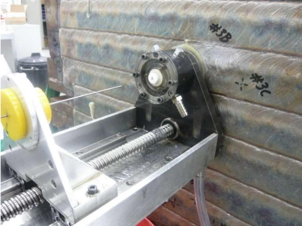
Figure 14 Gun drilling at location 3A during the iDHD measurements [30].
