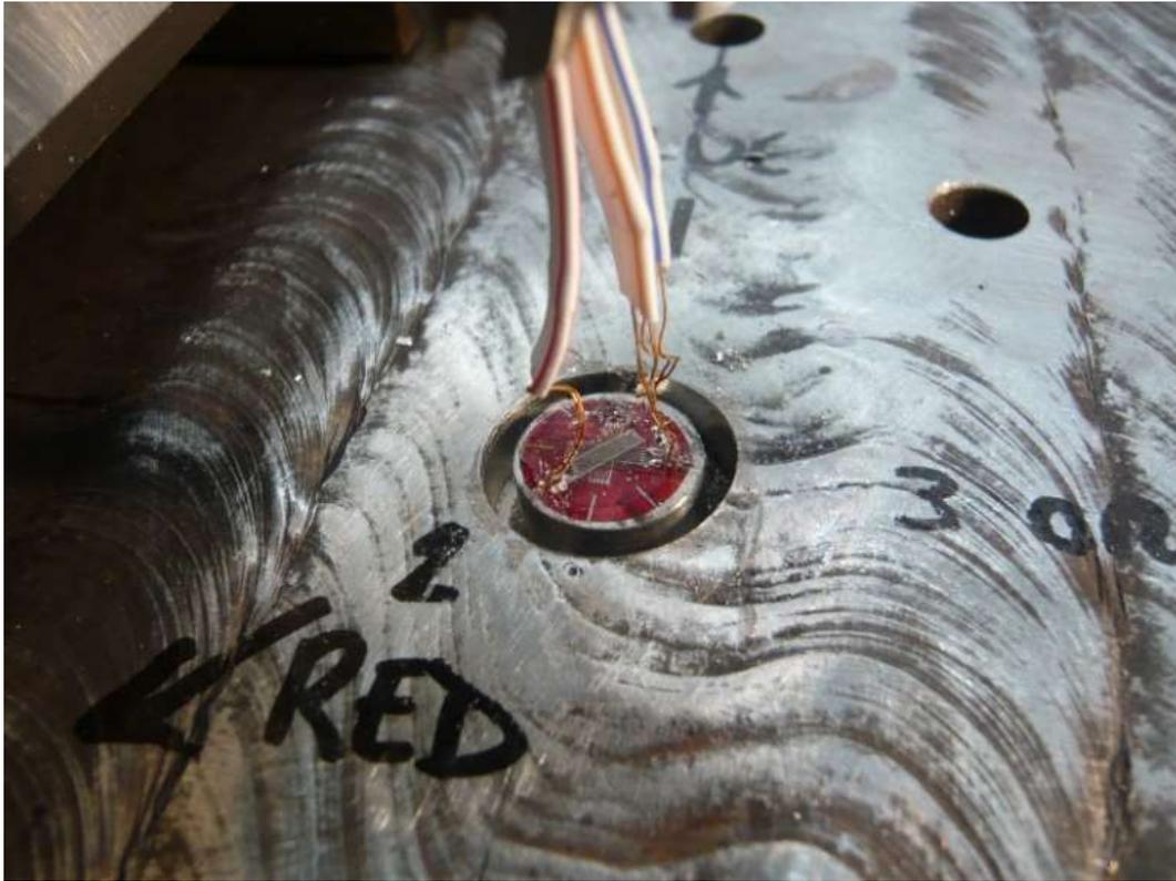
Figure 16 Strain gauge rosette and central core after RC measurement [30].
