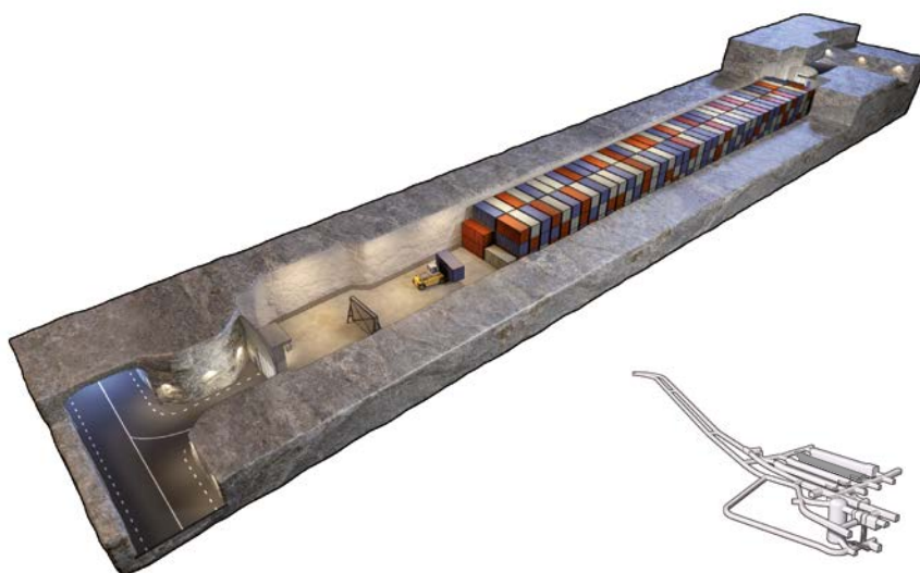
Figure 2-19. Vault for low-level waste, 1BLA, in SFR 1 during the operating phase.
