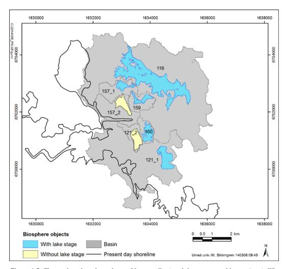
**Figure 6-7.** The resulting biosphere objects (blue or yellow) and their associated basins (grey). When the area is sea the basin is treated as the biosphere object, but thereafter the initial lake area (blue) is treated as the biosphere object. For the two objects that do not go through a lake stage (yellow), a wetland is formed directly after the sea stage.
