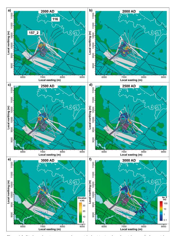
**Figure 6-1.** Discharge locations, expressed as particle densities (number of particles per m²), for particles starting in the SFR 1 rock vaults (left column, with SFR 1 pink shaded) and in the SFR 3 rock vaults (right column, with SFR 3 pink shaded), for time steps 2000 to 3000 AD (from Odén et al. 2014). White-contoured areas marked "116" and "157\_2" are included for orientation and indicate two of the SR-PSU biosphere objects (cf. below).
