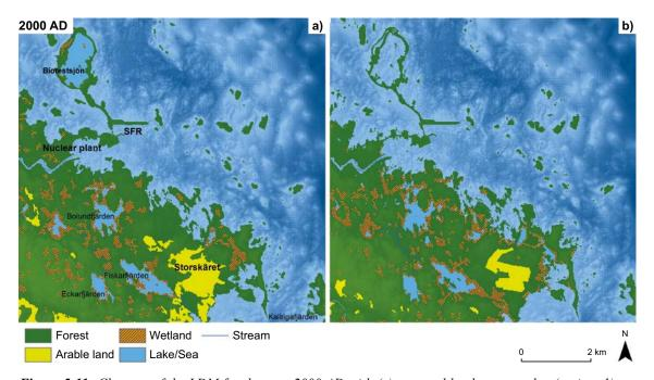
**Figure 5-11.** Close-up of the LDM for the year 2000 AD with (a) assumed land use as today (variant 1), compared with (b) the present map of Forsmark showing the distribution of five different ecosystems; see text for explanations to differences between the maps.
