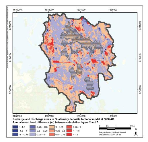
**Figure 4-7.** MIKE SHE-calculated annual average vertical hydraulic-head differences in the regolith at 5000 AD. Blue colours represent areas with upward flow (discharge) and red colours areas with downward flow (recharge). Dashed areas indicate the delineated biosphere objects (see Chapter 6).
