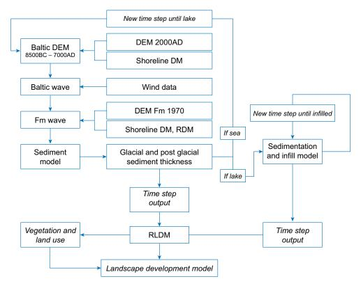
**Figure 5-3.** A conceptual flow chart of the coupled regolith-lake(-biota) development model (RLDM). The flow chart describes the work process and the linkage between the underlying models used for each time step to build the landscape development model (LDM) for Forsmark ("Fm" in the figure). The marine module runs independently from the lake module and the lakes are modelled separately depending on their appearance in time.
