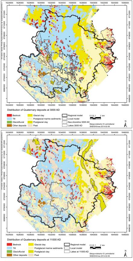
Figure 4-6. Surface distributions of regolith at 3000 AD (top) and 11,000 AD (bottom), according to the modelling with the regolith-lake development model, RLDM (Brydsten and Strömgren 2013). The areas indicated on the map are the regional (thick black line) and local (grey line) model areas used in the hydrological modelling (Section 4.4.1). The brown areas mark man-made deposits within industrial areas, i.e. the nuclear power plant to the west and the Forsmark harbour with the SFR facility.
