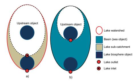
**Figure 6-4.** Conceptual illustration of sea-lake-terrestrial type object. a) Two lake objects in a catchment where the bottom lake object has a sub-catchment defined by the outlet catchment area minus the inlet catchment area, and the lake watershed area equals the total lake catchment including upstream objects. b) The basin is the area defined by the catchment of the lake outlet minus the catchment of any upstream object.
