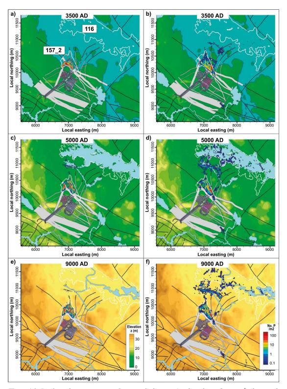
**Figure 6-2.** Discharge locations, expressed as particle densities (number of particles per m²), for particles starting in the SFR 1 rock vaults (left column, with SFR 1 pink shaded) and in the SFR 3 rock vaults (right column, with SFR 3 pink shaded), for time steps 3500 to 9000 AD (from Odén et al. 2014). White-contoured areas marked "116" and "157\_2" are included for orientation and indicate two of the SR-PSU biosphere objects (cf. below).
