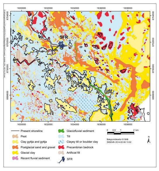
**Figure 3-3.** Surface distribution (at a depth of 0.5 m) of regolith and areas with exposed bedrock in the Forsmark area. Note that lakes and the sea are shown without surface water.
