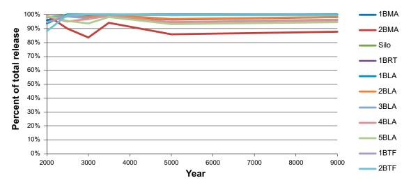
**Figure 7-3.** Fractions (%) of total potential release from the repository parts that reach the biosphere in object 157\_2 over time, average of 17 hydrogeological realisations.
