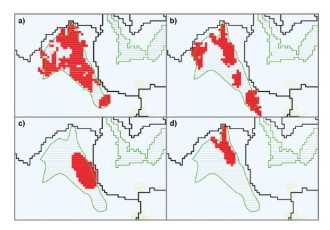
Figure 6-14. Alternative delineations of biosphere object 157\_2. The green line indicates the original object and the red areas the alternative outlines of the biosphere object. a) Areas with upward hydraulic gradients (from bedrock to surface). b) Wetland areas (water above surface or not deeper than 0.25 m below the surface). c) Area with a high density of repository discharge points at the bedrock-regolith interface. d) Potential area for cultivation, after drainage of mire.
