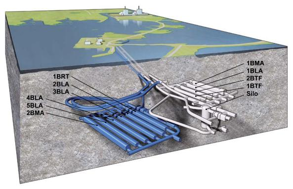
**Figure 2-1.** Illustration of the SFR repository. White represents the existing repository SFR 1, and blue is the planned extension SFR 3. The tunnels to the repository extend to the surface buildings (centre of picture). The dimension and functions of the rock vaults (BMA, BLA, BTF and RTF) and Silo and the different types of waste are described further in the **Initial state report**.
