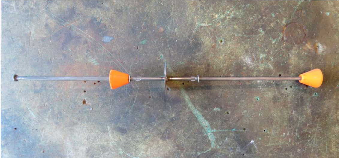
Figure 4-2. Example of form rods.
